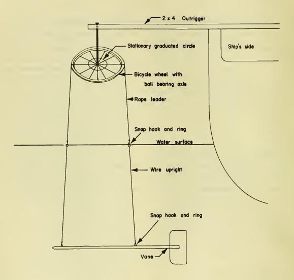
Figure 3. -- Subsurface current-direction indicator.
