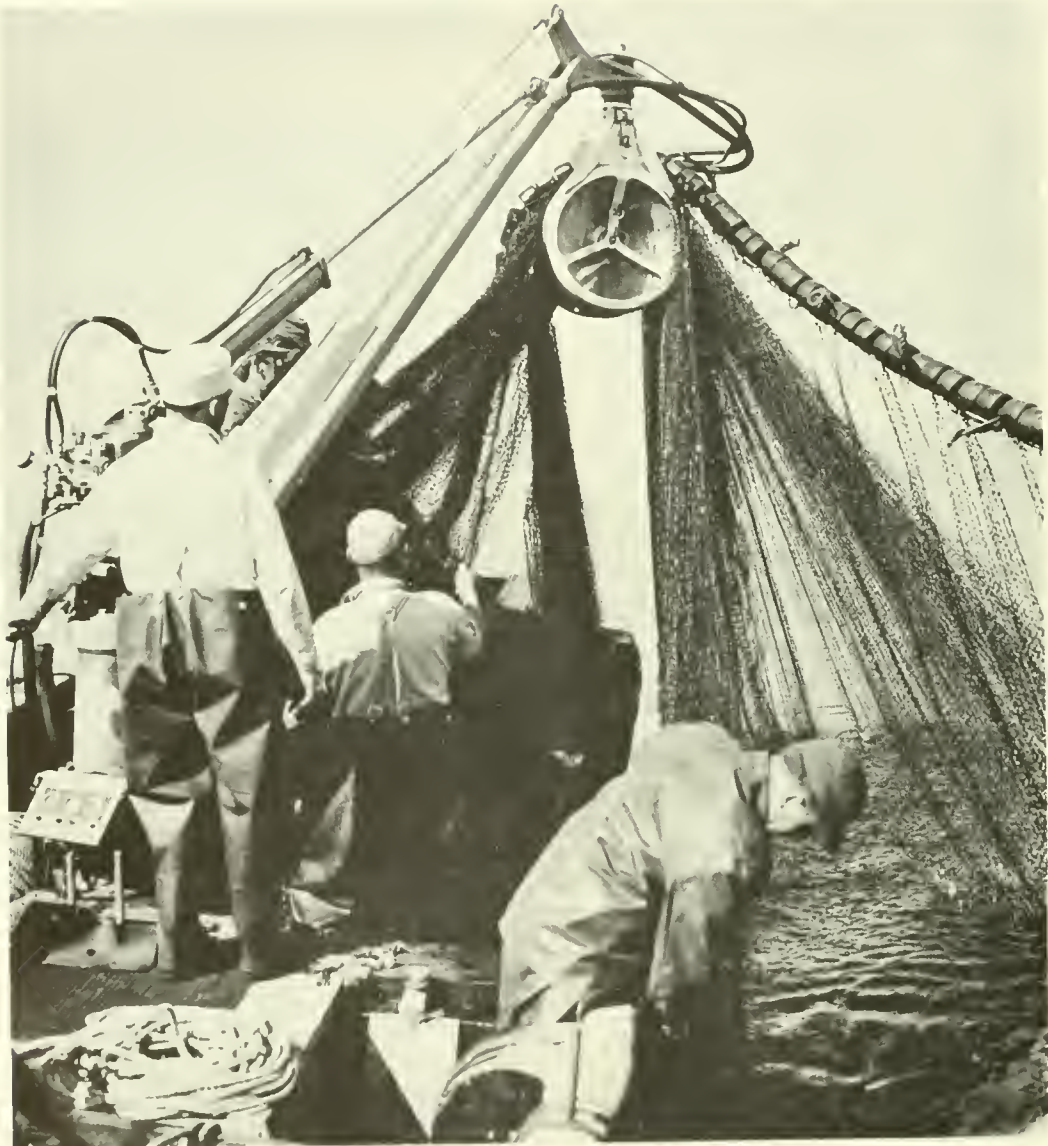
Figure 2.--Net-handling equipment mounted on a menhaden seine boat.
