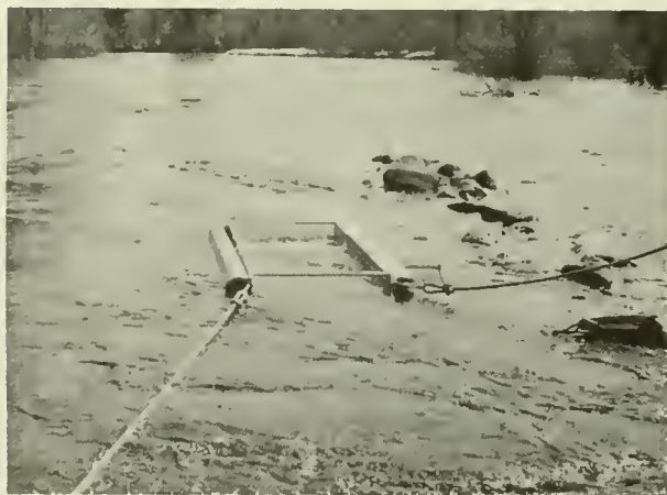
Figure 10.--Scoop-type migrant trap used for capturing young fish in the Wenatchee River. (Design and plans courtesy Washington Department of Fisheries)
