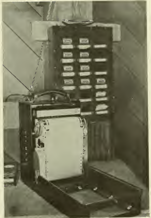
FIGURE 8.--OPERATIONS RECORDER USED TO RECORD FISH PASSAGE IN NUMBERS PER UNIT TIME. EACH PASSAGE IS NOTED IN THE FORM OF A BLIP ON THE RECORDER TAPE AT THE EXACT MOMENT OF OCCURRENCE.
