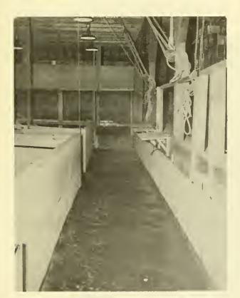
Figure 4.--Main tank with a 5-foot channel used in a study of the effect of sonic tags on swimming ability and behavior of adult salmonoids.
