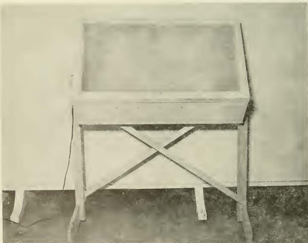
Figure 6.--Lightbox for viewing X-ray films of menhaden vertebrae.
