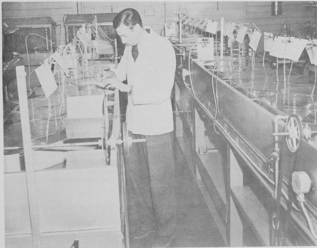
FIGURE 1. Constant temperature troughs utilized in the screening program. Concurrent tests of 48 different substances are shown in progress. Routine observations are being noted on the individual test record cards.
