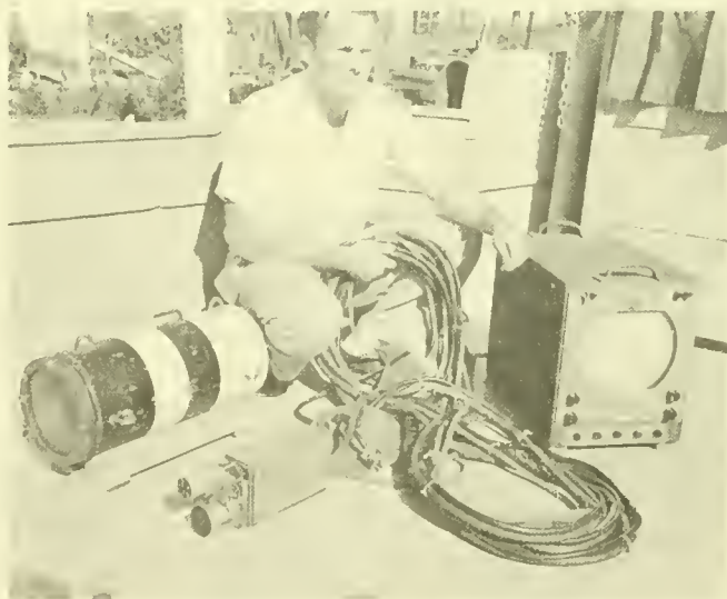
Fig. 6. Underwater-Television chain. Left to right- camera pressure vessel, T-V camera, multi-conductor cable and control monitor.
