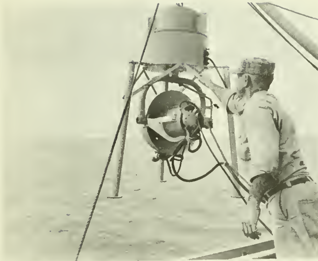
Fig. 8. Rear view of Underwater Television shows tripod legs, pressure vessels, camera cradle and cable attachments for underwater photo-flood lamp. Arrow indicates vertical drive linkage which operates vertical scanning.
