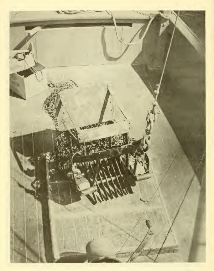
Fig. 3. Hard-shell clam dredges are operated from 30 - 1/5 foot power boats in the southern half of the Sakonnet River.
