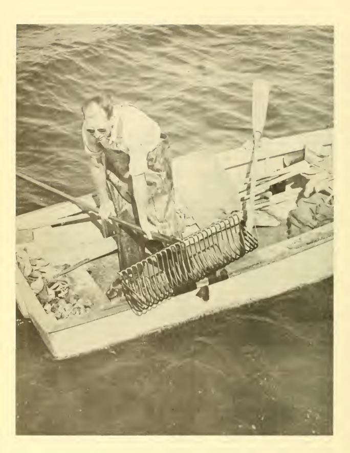
Fig. 2. Bullrakes are used by about half of Rhode Island's 1,400 "hand" diggers.
