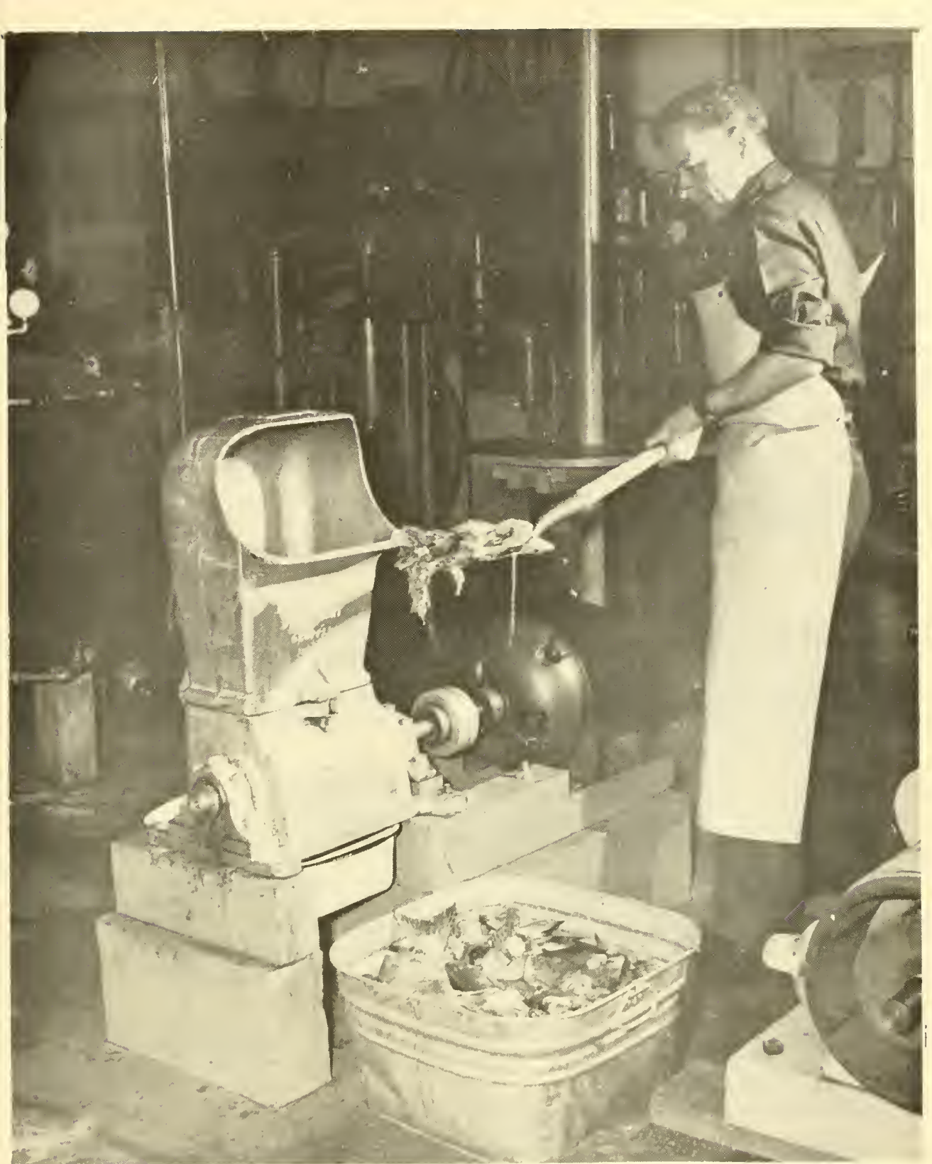
PLATE 4. - GRINDING SALMON WASTE IN HERCULES MEAT- BONE CHOPPER FOR PREPARATION OF HATCHERY FEED.
