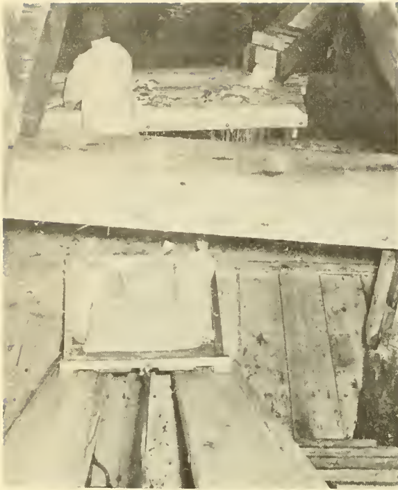
Figure V-6. The sacks of viscera are loaded onto the elevator and are hand-winchd from the platform up to the dock level.
