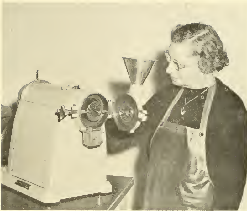
Figure II-1. Attrition-type mill used to grind dry materials such as fish meal samples.
