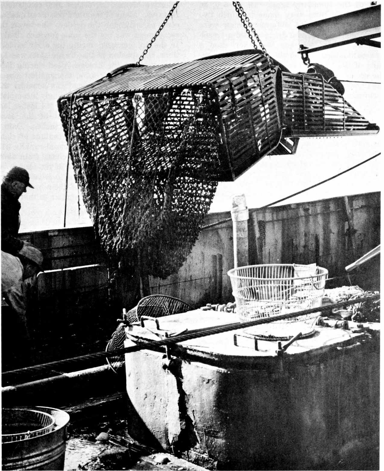
Figure 5.—Complete hydraulic jet dredge as viewed from the stern. The bag and the cage (to which the bag is attached) were submerged in Figure 3. Note the “blade” of the dredge extending below the runners of the dredge. The blade is spring-mounted and will ride over the surface of the bottom when the dredge is being towed with the jets turned off. When the jets are on and cutting a trench, the blade will follow and retain contact with the bottom of the trough.
