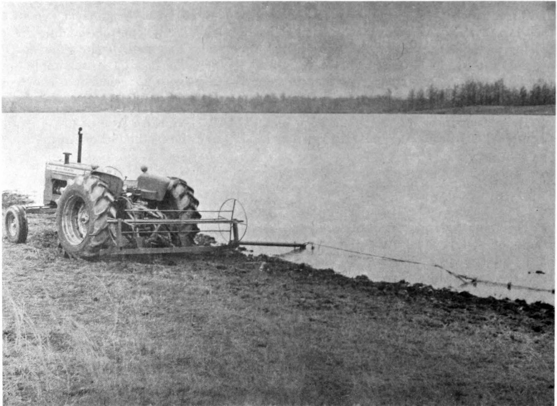
Figure 2.—Tractor mounted tow bar (with net reel) attached to a seine in a commercial catfish pond.
