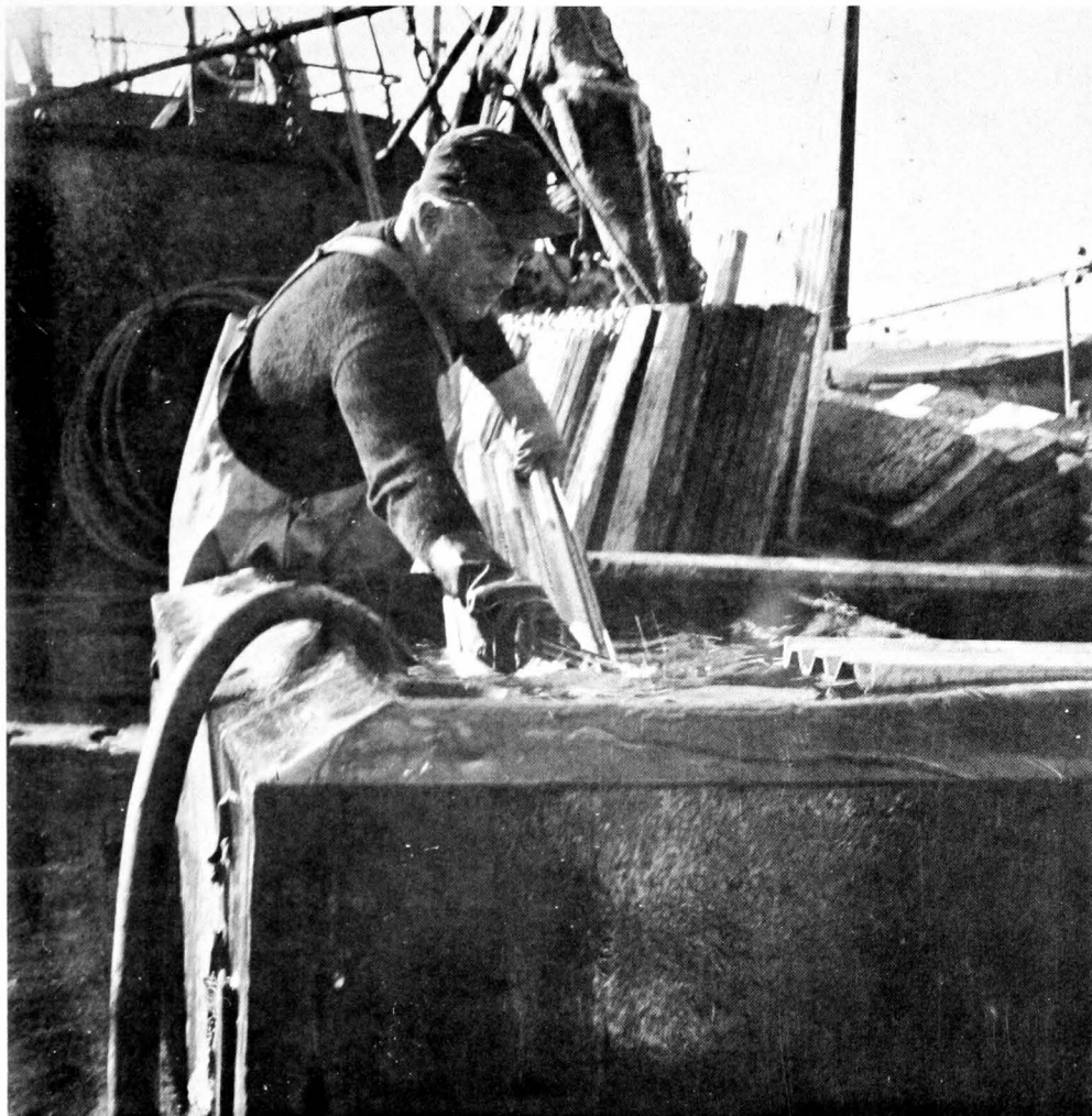
Figure 9.—Washing penboards. Boards are stacked on deck after washing to permit drying before they are reused in the fish hold.
