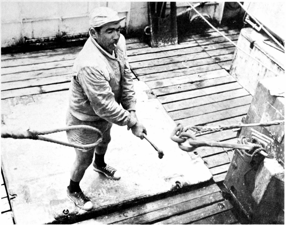
Figure 2.—“Let go!” At this command, marking the start of a set, a crewman strikes the pelican hook release, dropping the seine skiff into the water. (Photo taken aboard Jeanne Lynn .)
