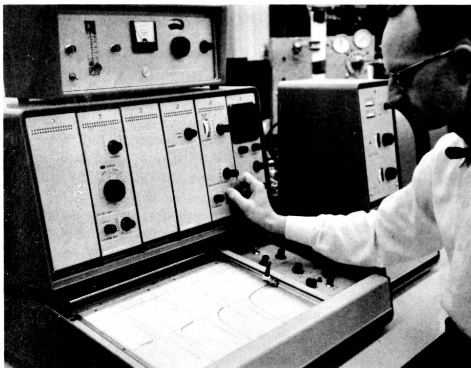
Figure 1.—Electron paramagnetic resonance spectrometer. The microwave generator and electromagnet are located in the module at the far right.
