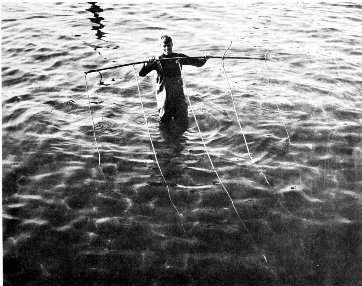
Figure 3.—Laboratory electrode array being set up at the test site in St. Andrews Bay, Florida.
