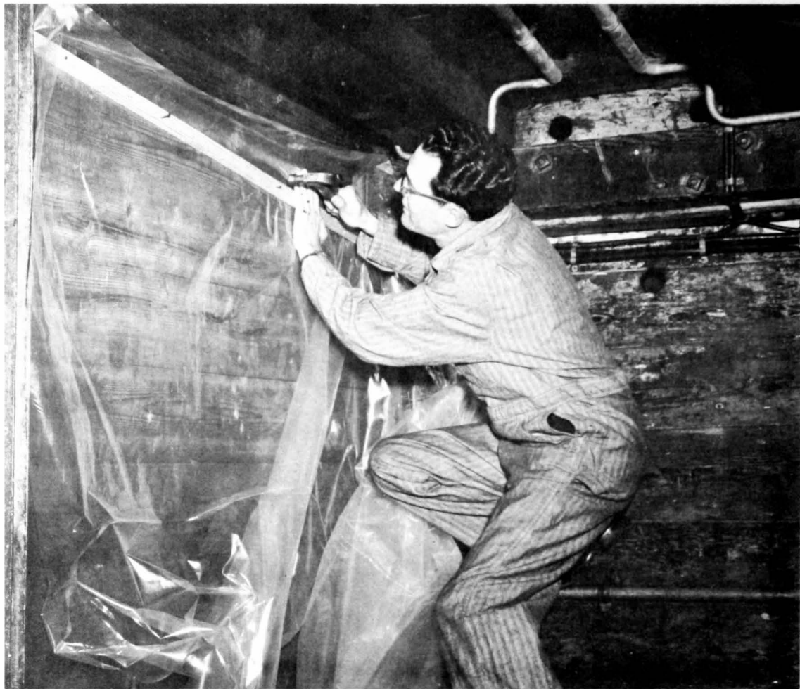
Figure 2.—Lining a dry pen in the hold of a halibut vessel before ice is taken on.
