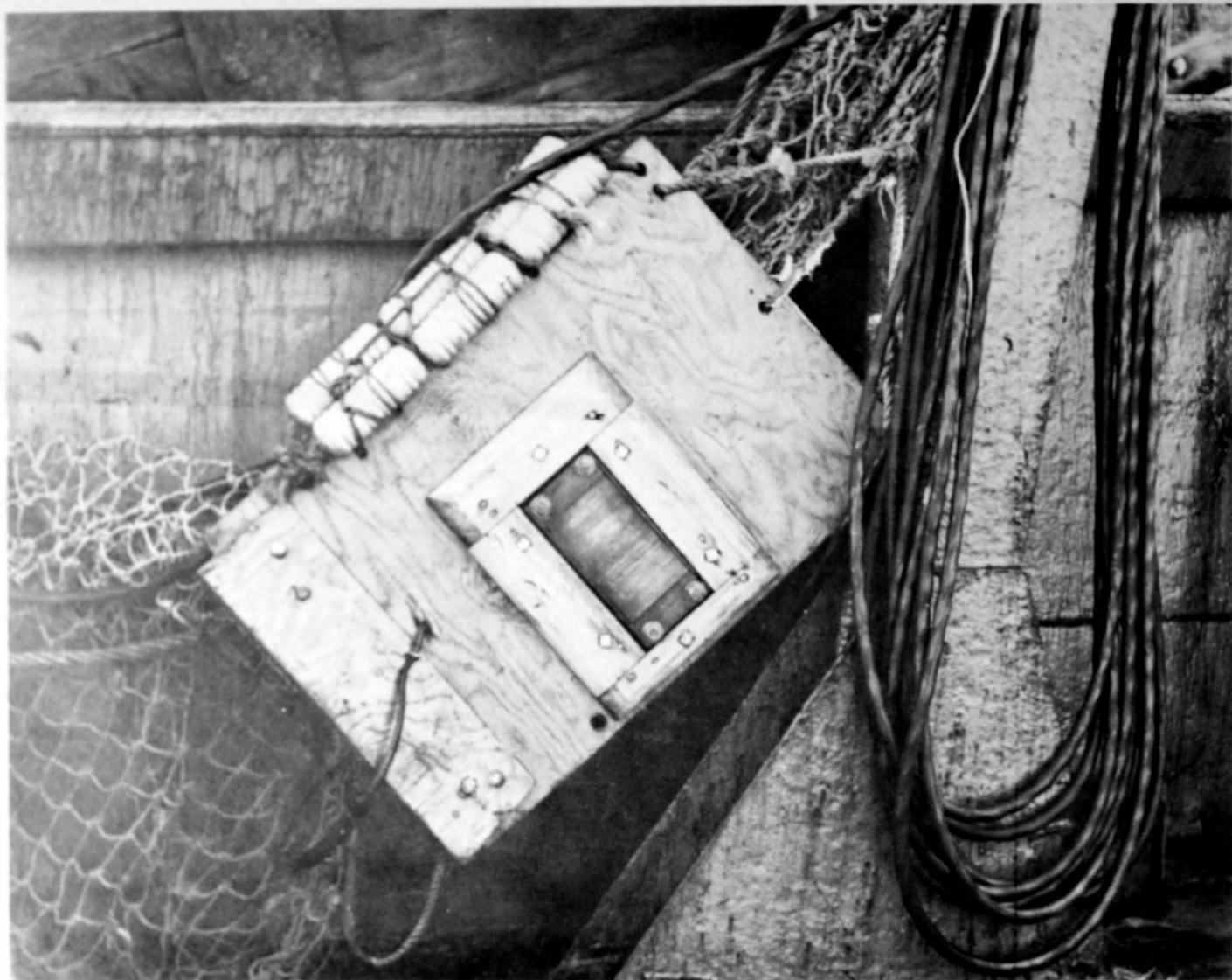
Figure 4.—Net wing-end sonic transducer. The transducer is mounted within a polyester resin-covered wooden framework. A similar transducer is attached to the opposite wing.
