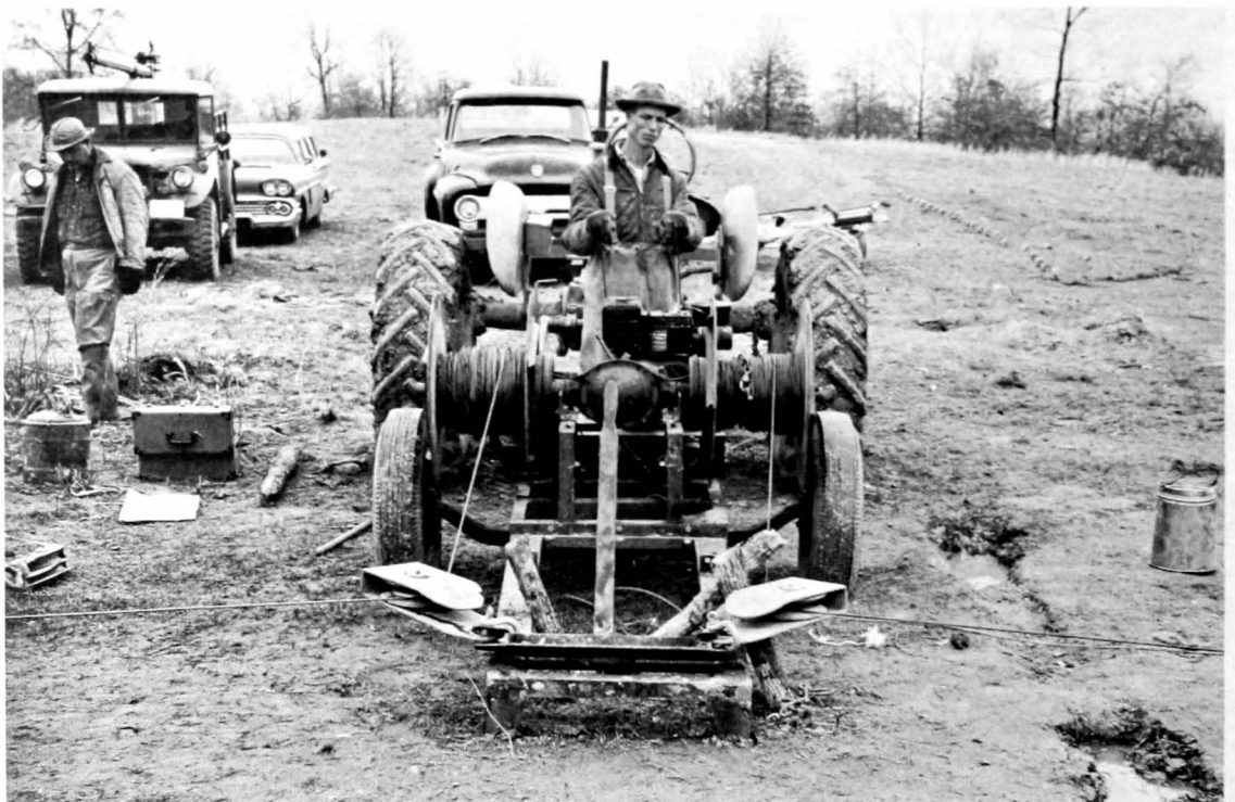
Figure 5.—Bureau-designed haul seine puller, using cable for hauling lines. Earlier tests were made with the puller mounted on a trailer.
