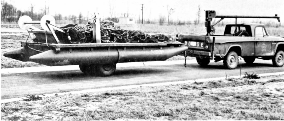
Figure 4.—Mobile pontoon barge used for hauling and setting farm-pond haul seine.
