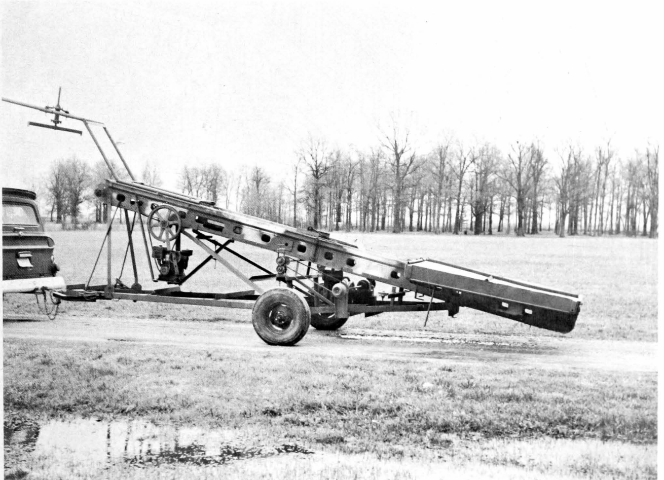
Figure 6.—Seine puller mounted on support frame beneath fish conveyor, combining seine puller and conveyor into single compact unit.
