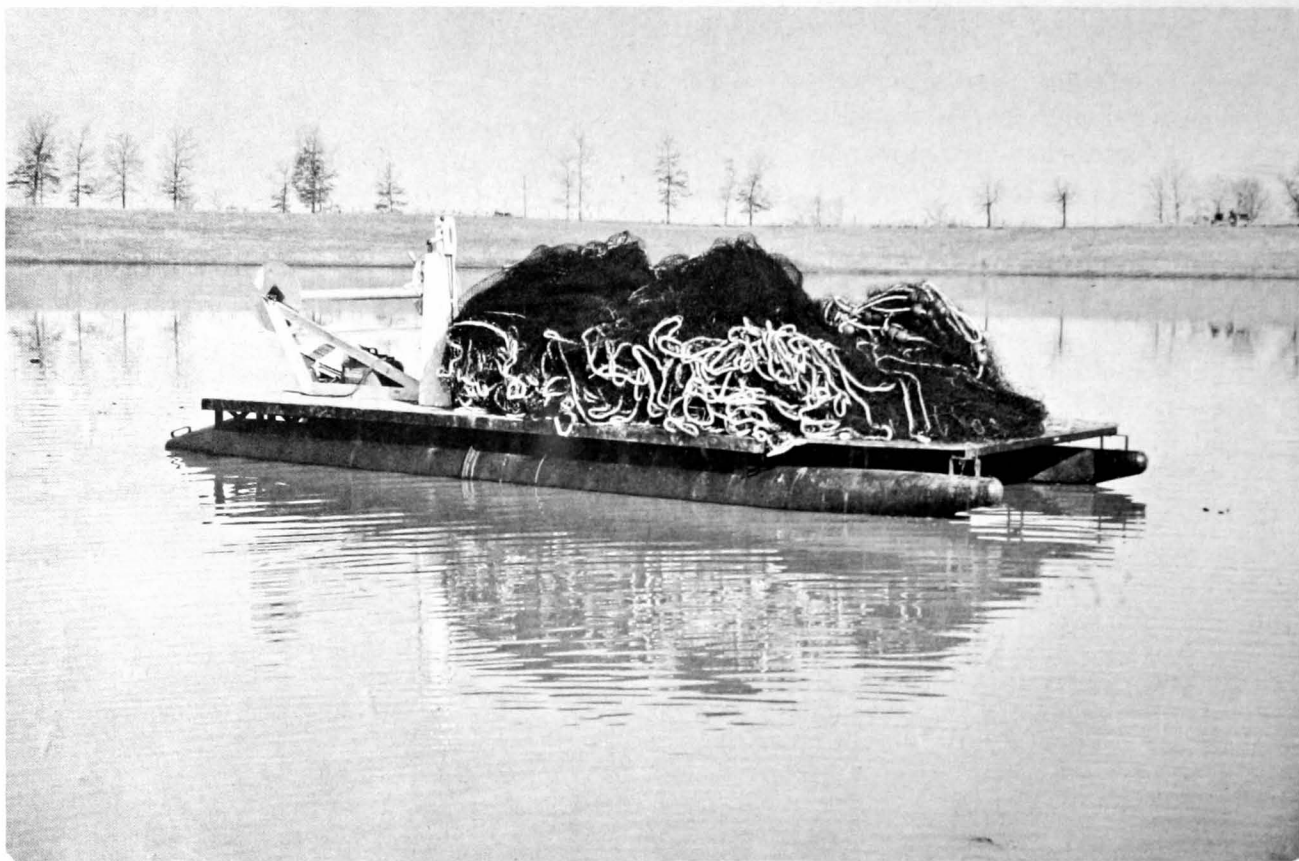
Figure 11.—Nylon haul seine stacked on pontoon barge and ready to be set over the stern roller.
