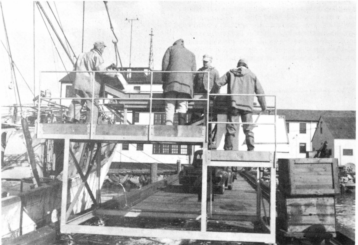
Figure 4.--Fish-Handling Unit Number IV being used for unloading fish from the Delaware .
