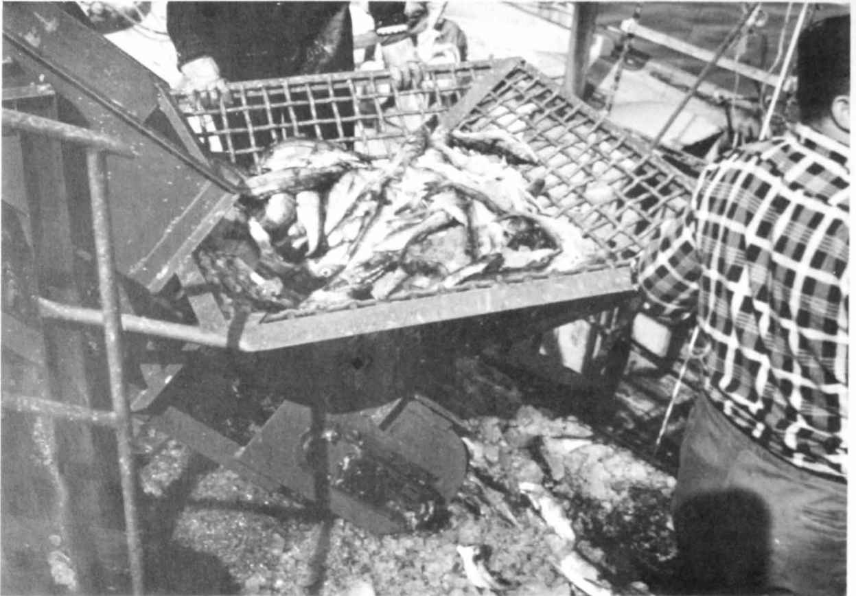
Figure 6.--Receiving hopper of Fish-Handling Unit Number V during tests at the State Fish Pier in Gloucester, Mass.
