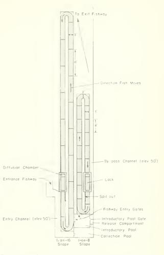
Figure 10.—Plan view of the 1-on-16- and 1-on-8slope endless fishways with auxiliary approach channels and pools.
