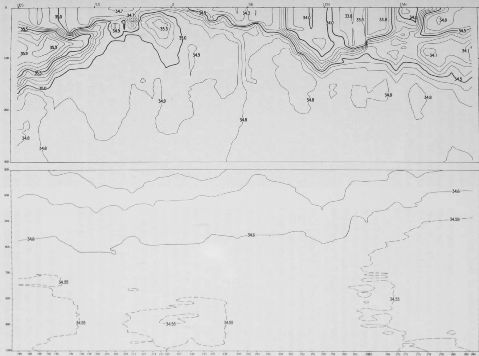
Figure 6.—Computer-drawn vertical section of salinities from STD data taken aboard the National Marine Fisheries Service RV David Starr Jordan on EASTROPAC Cruise 12 along long 112° W from lat 20° N to 10° S during February 1967. Isotherms, chart borders, and labels were constructed in the computer and drawn by CalComp Plotter. A draftsman relabeled and widened every fifth contour.
