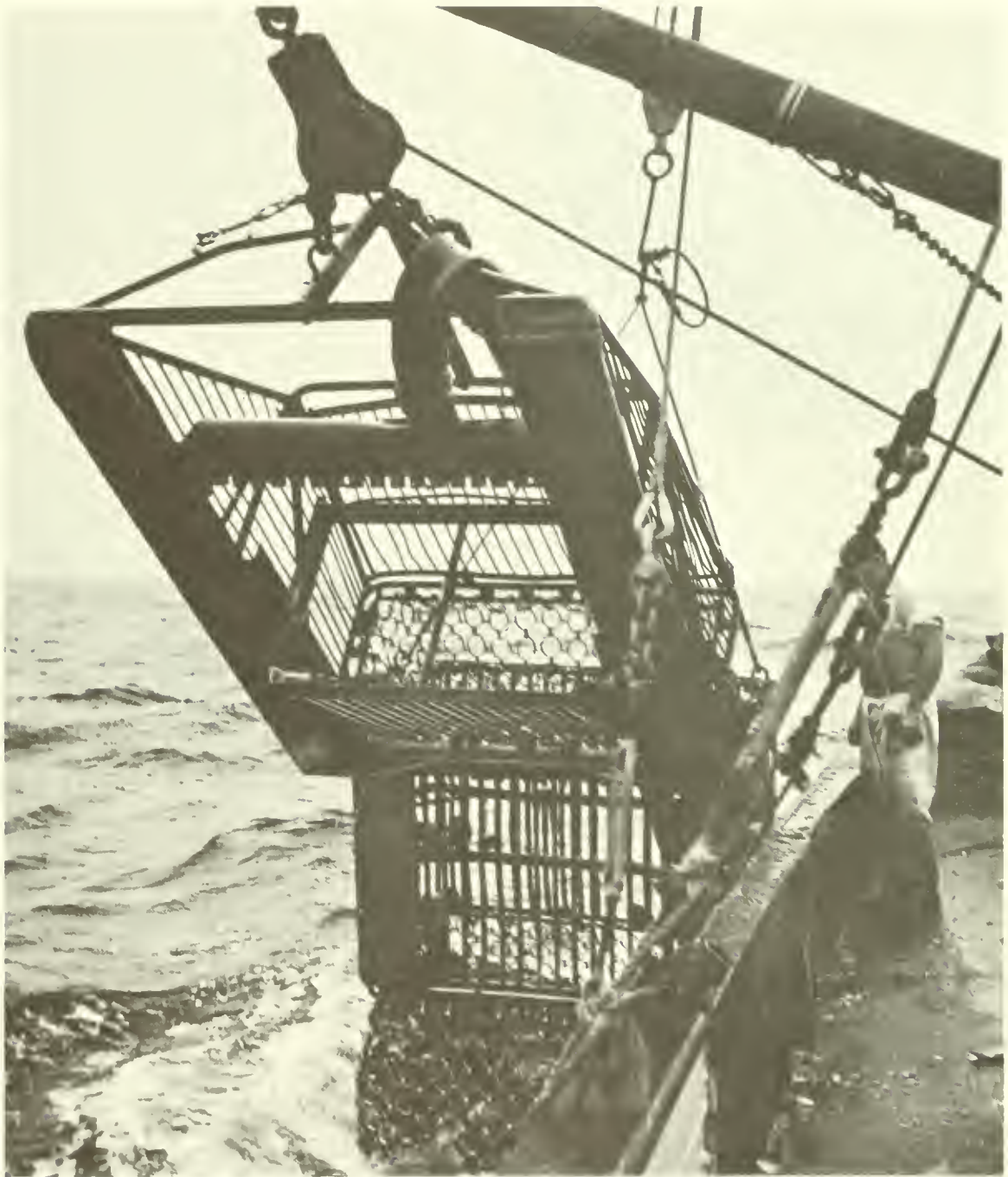
Figure 7.—Classic 40-inch hydraulic jet dredge used by the majority of fishing vessels operating along the coast of New Jersey and Maryland during the late 1950's and up to the present time. Note that the dredge itself is all enclosed except for the bottom and forward section of its top. Loose aprons built out of rings are used to enclose the space between the dredge and sled to prevent loss of clams between the two units. In addition, chain attachments are used between the two units for towing purposes. Attached to the sled is the chain bag built of 3-inch scallop rings and connectors. This dredge is equipped with a straight edge knife. Many dredges use a V-shaped knife that floats on springs and digs into the bottom only after the water to the jets is turned on. In use of spring-mounted blades, the knife settles into a trough which is jetted out by the water. Dredges with this type of blade also use a V-shaped manifold as compared to the straight manifold shown here. The clam jetting hose shown has been built especially for clam jetting and has a 5-inch inside diam.
