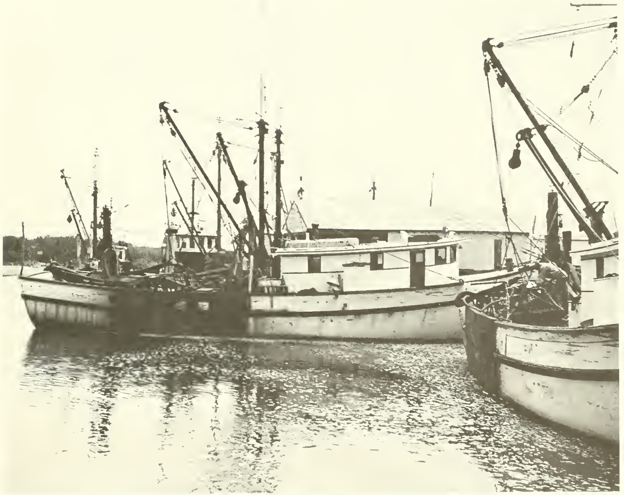
Figure 15.—A converted shrimp boat. One of the several different vessel types which were converted for surf clam dredging.
