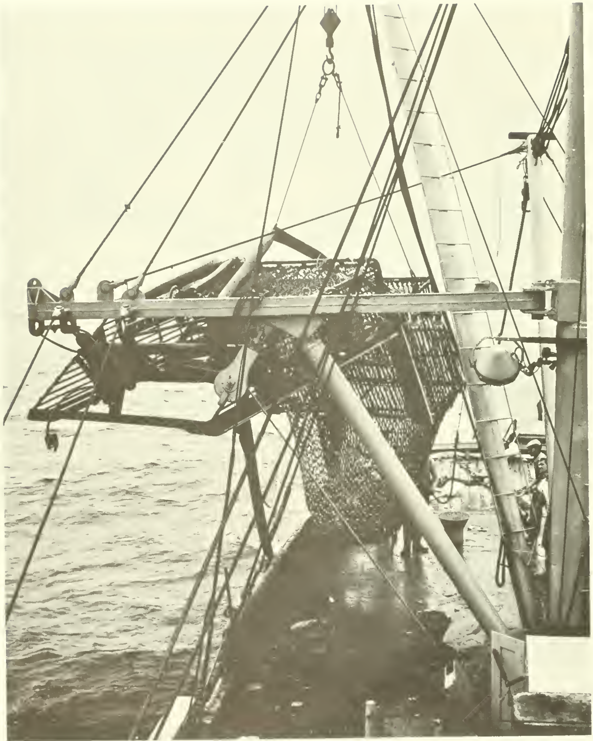
Figure 5.—Photograph of largest hydraulic jet dredge in use today by the surf clam industry. This is an 84-inch dredge used aboard the 136-ft Gail Borden . Note size of auxiliary gear and deck equipment required for the operation of this size dredge. Two 6-inch inside diam. water supply hoses are required for the jetting action of this dredge on the bottom.
