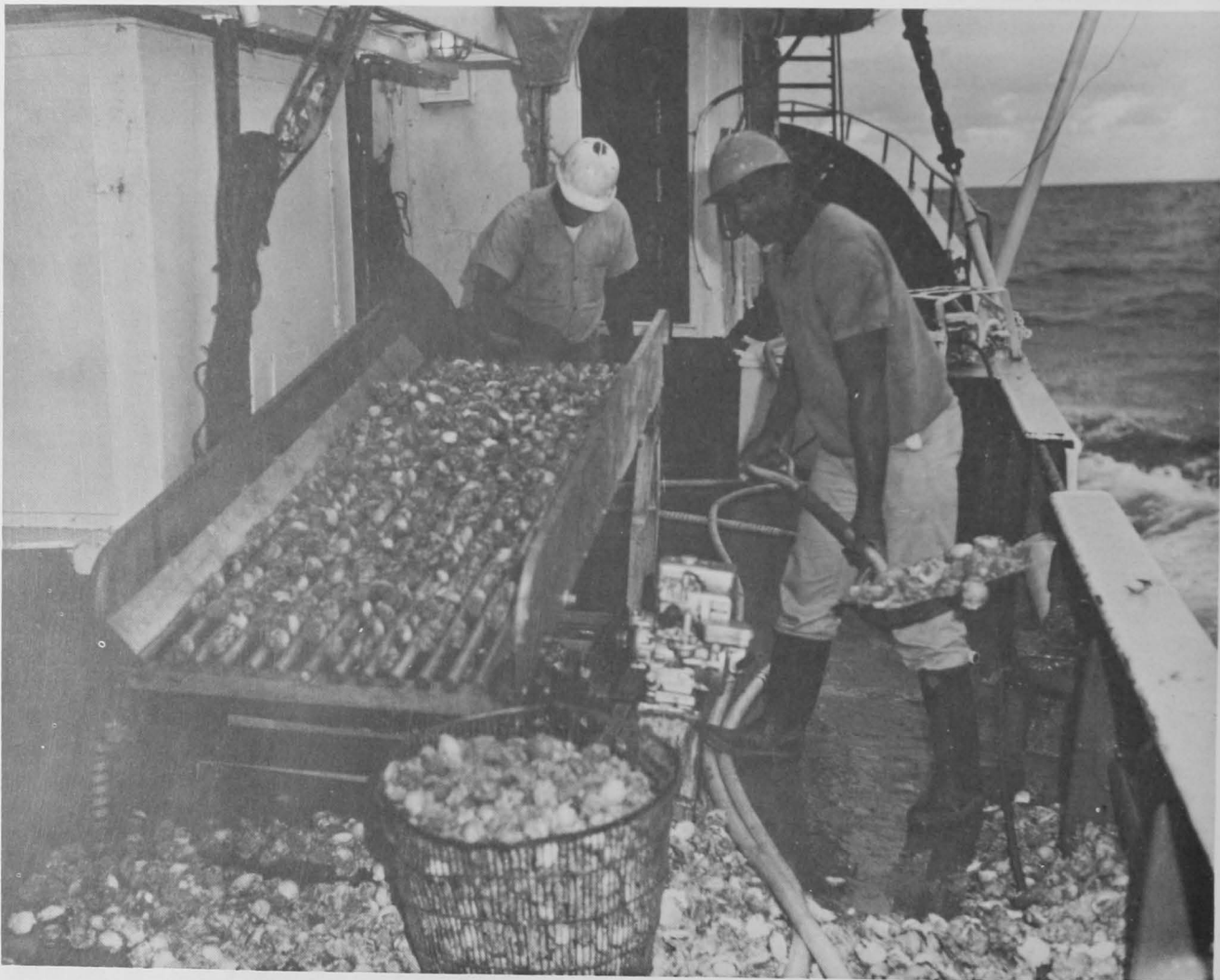
Figure 26.—Testing an industry-designed calico scallop culler on the Oregon .
