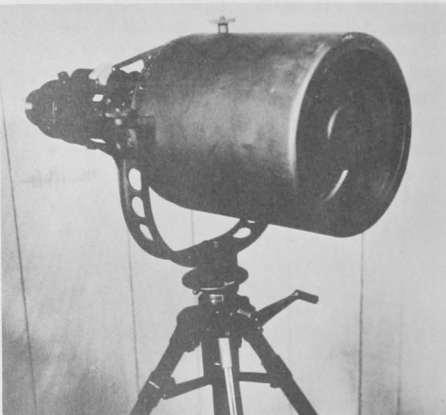
Figure 9.—Image intensifier (night observation device) specially designed for airborne observations. The device amplifies bioluminescence 75,000 times that seen with the naked eye.
