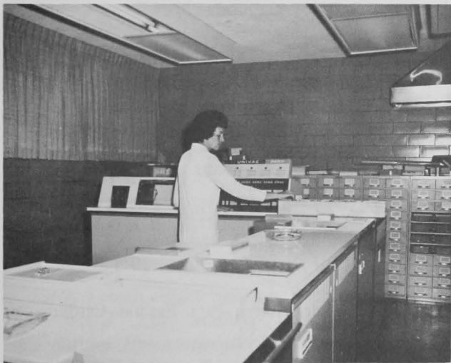
Figure 27.—The UNIVAC 9200 computer used to process exploratory fishing data.
