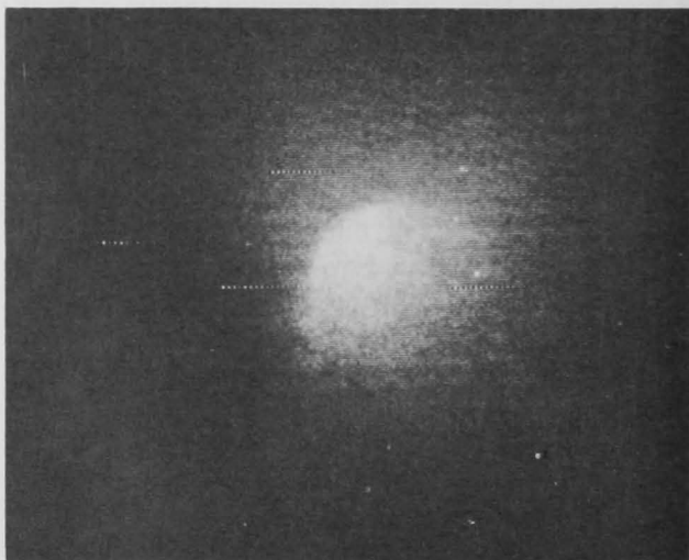
Figure 10.—School of Atlantic thread herring, Opisthonema oglinum , detected at night from an altitude of 3,500 feet. The bioluminescent image is caused by school's movement through the water. This television screen photograph shows the faint glow amplified 55,000 times by the image intensifier.
