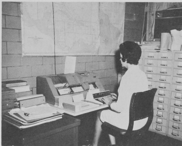
Figure 28.—Technician keypunching data cards in the Exploratory Data Center.
