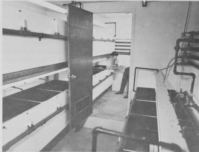
Figure 9.—Sea-water laboratory designed for rearing menhaden from eggs through the postlarval stage.
