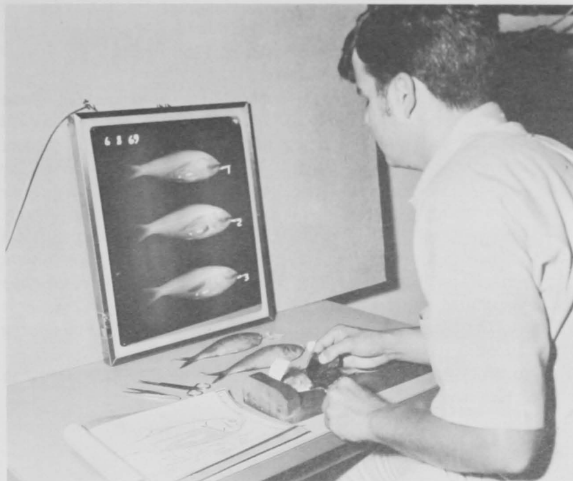
Figure 15.—Technician determining the location of tags in menhaden recovered with an electronic detector system. Tags and pins marking the approximate point of tag insertion on fish that have not healed can be seen.
