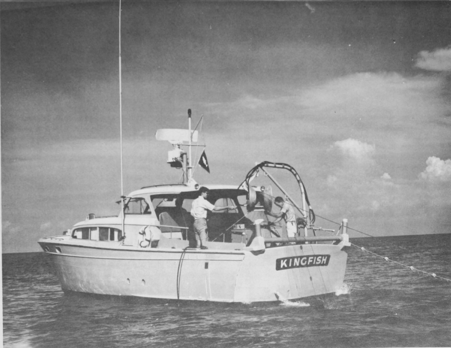
Figure 20.—R/V Kingfish rigged with a powerblock for sampling thread herring with monofilament gill nets.
