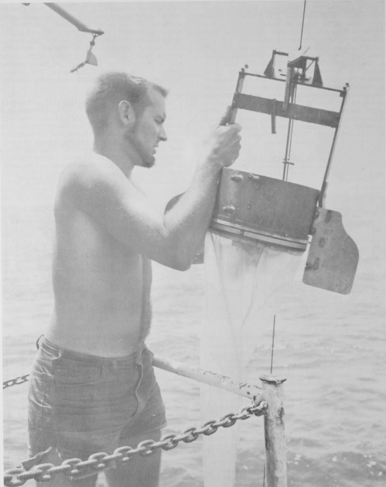
Figure 47.--A BCF oceanographer (aboard the Geronimo ) attaches a Clarke-Bumpus plankton sampler to a towing wire on Equalant cruise II in the Gulf of Guinea.
