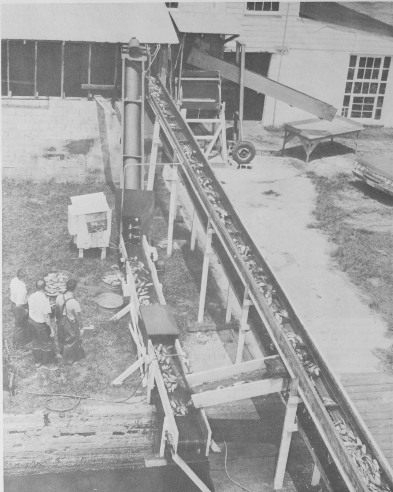
Figure 4.--Prototype electronic detector system at Seashore Packing Co., Beaufort, N.C. A portion of the catch being conveyed to the plant by a dragline (right) is diverted onto a high-speed belt conveyor. As a tagged fish passes through the detector, a door is activated to push the fish off the belt into a tub. The remaining fish pass up the screw conveyor and are returned to the dragline.
