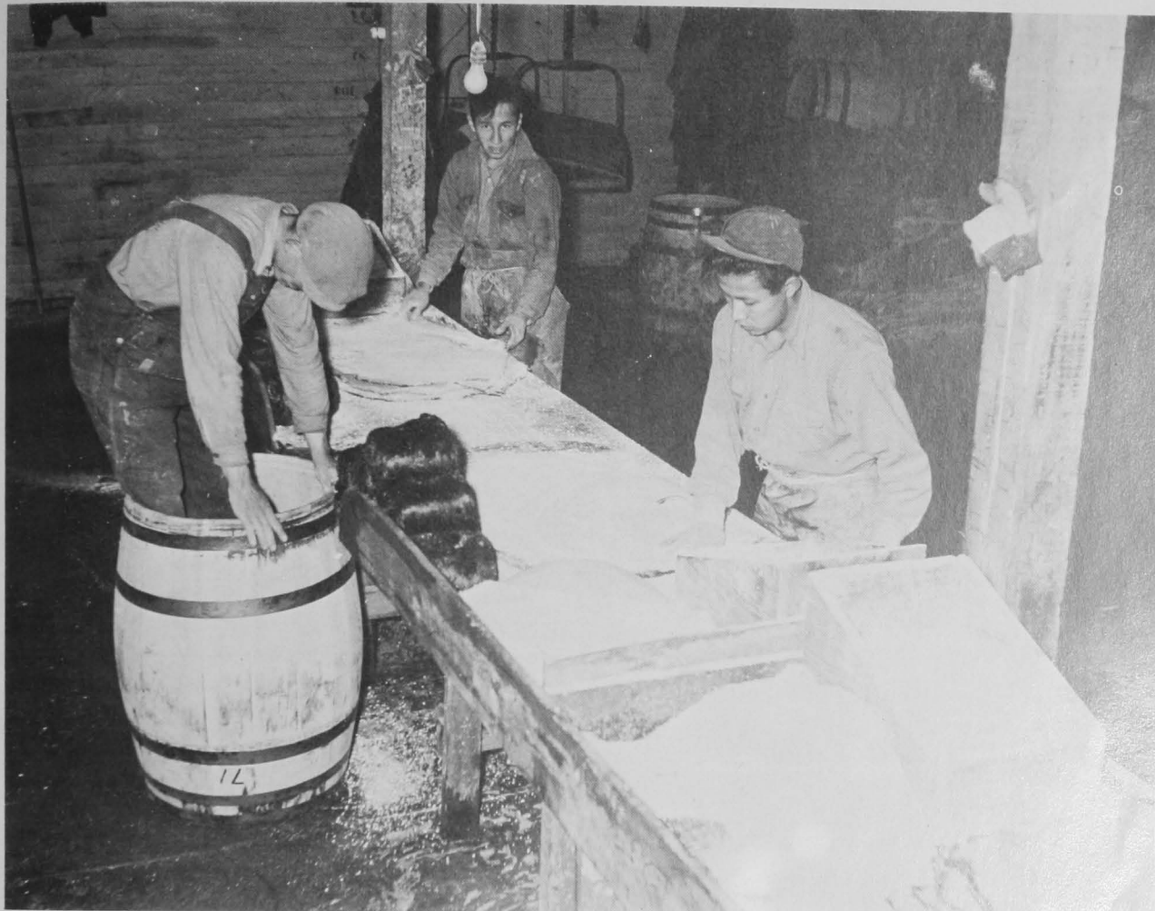
Skins that have been washed, cleaned of blubber, cured in a saturated salt solution, and drained are rubbed with salt and boric-acid powder, rolled, and tightly packed in barrels for shipment.
