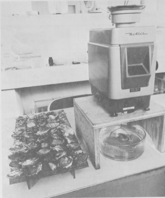
Figure 18.--Oysters are weighed suspended in water.
