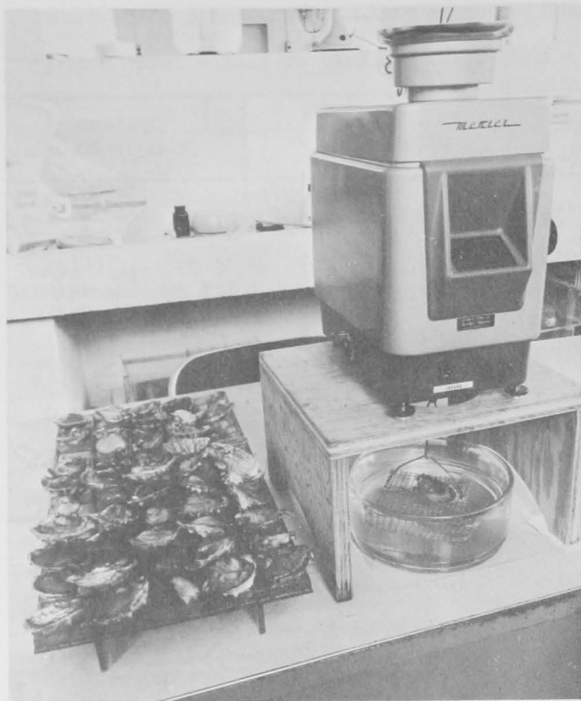
Figure 18.--Oysters are weighed suspended in water.
