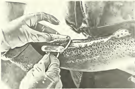
FIGURE 28.—Sonic tag being attached to 7-pound steelhead trout. One capsule contains mercury cell battery and 70-kHz transducer; adjoining capsule houses oscillator circuit components. Transmitting range is 1 to 2 miles in fresh water, or about 1 mile in salt water. Battery life is 10 weeks.
