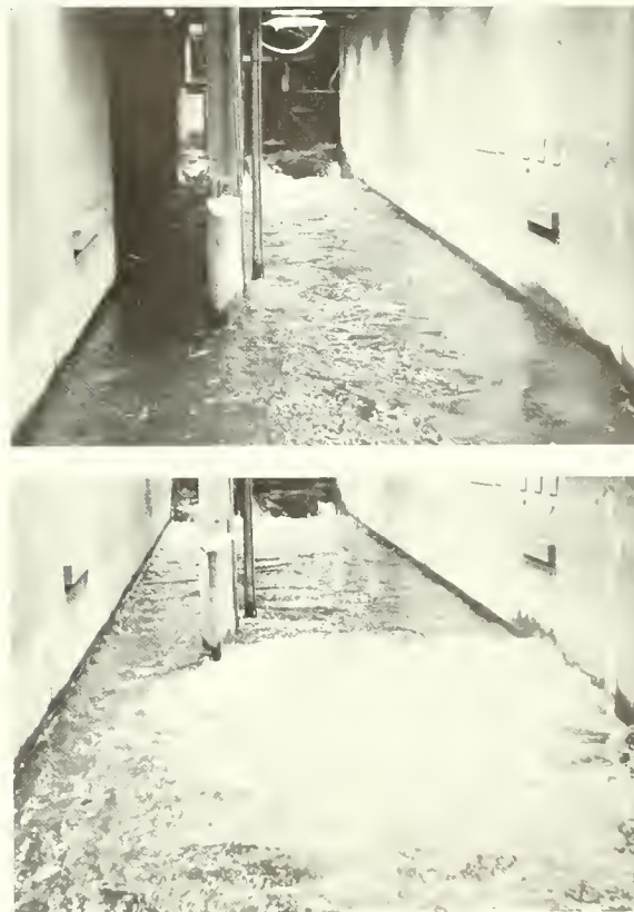
FIGURE 26.—TOP. Testing the response of fish to illuminated and dark channels at Bonneville Dam. BOTTOM. Fish were reluctant to pass through a screen of air bubbles.
