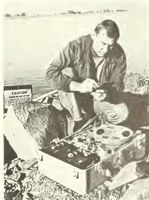
FIGURE 30.—Shore monitor which records passage of sonic-tagged fish. Data include date, hour, direction of passage, and repetition of tag pulses. Variations in the latter indicate where and when fish was tagged. Monitor is completely automatic; units need servicing only once every 7 to 10 days.
