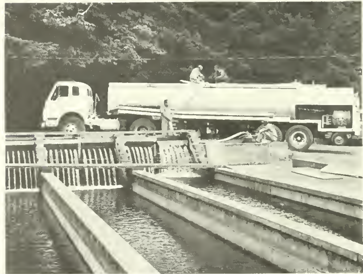
FIGURE 40.—Truck used to transport fingerlings around dams. The 5,000-gallon tank truck has a refrigeration-aeration system and filter. Capacity is 400,000 fish, 2½-inches long.
