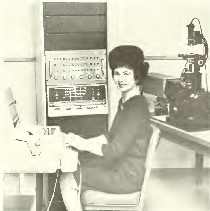
FIGURE 18.—Experimental operation of semiautomatic machine for reading fish scales. Image of scale under microscope (right) is fed to computer (center). The computer analyzes the light and dark areas of the scale and results are printed on teletype (left).
