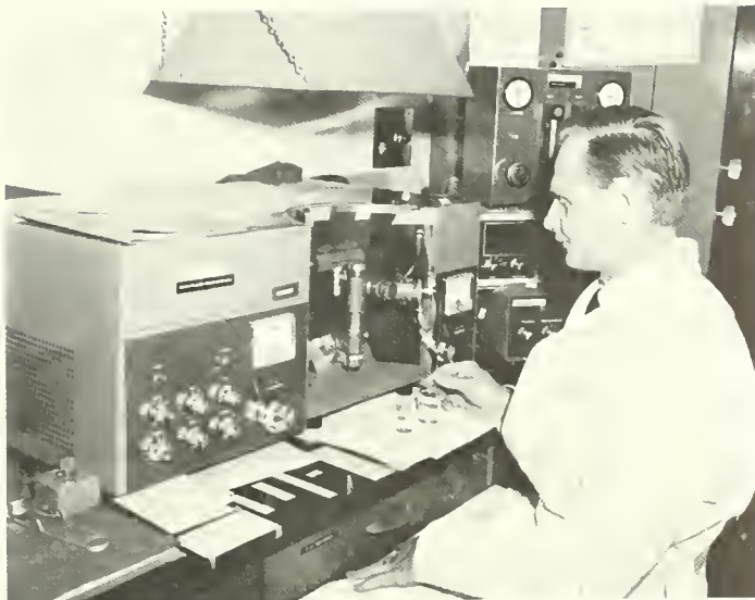
FIGURE 12.—Measurement of trace element content of sea water by atomic absorption spectrometry.
