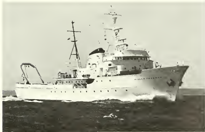
FIGURE 5.—Bureau's newest research vessel, the 215-foot Miller Freeman was launched in 1967. She carries 9 scientists and a crew of 28. Her cruising speed is 14 knots, and maximum range is 16,000 miles.
