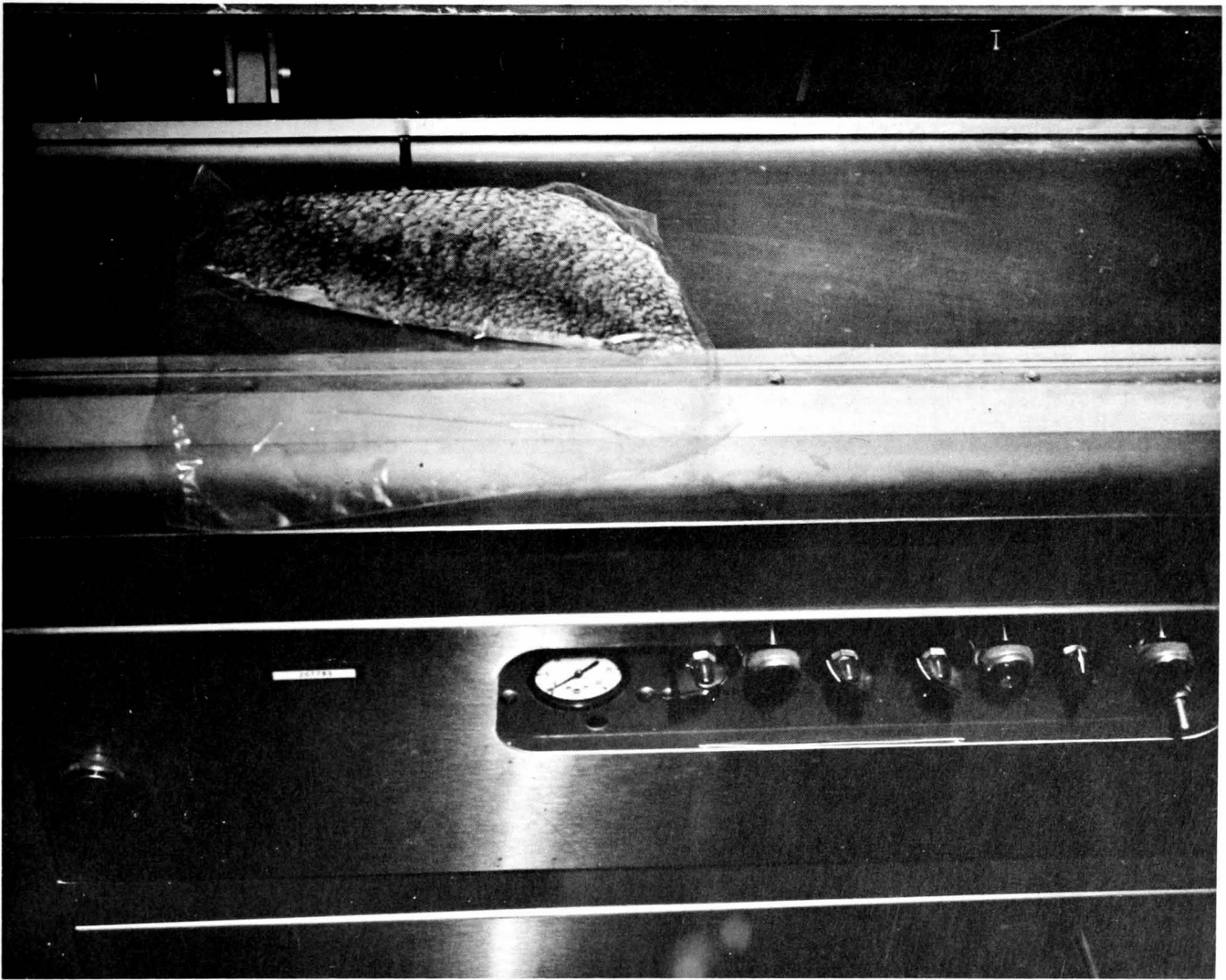
Figure 1.--Processing snapper in vacuum bags to prevent browning.
