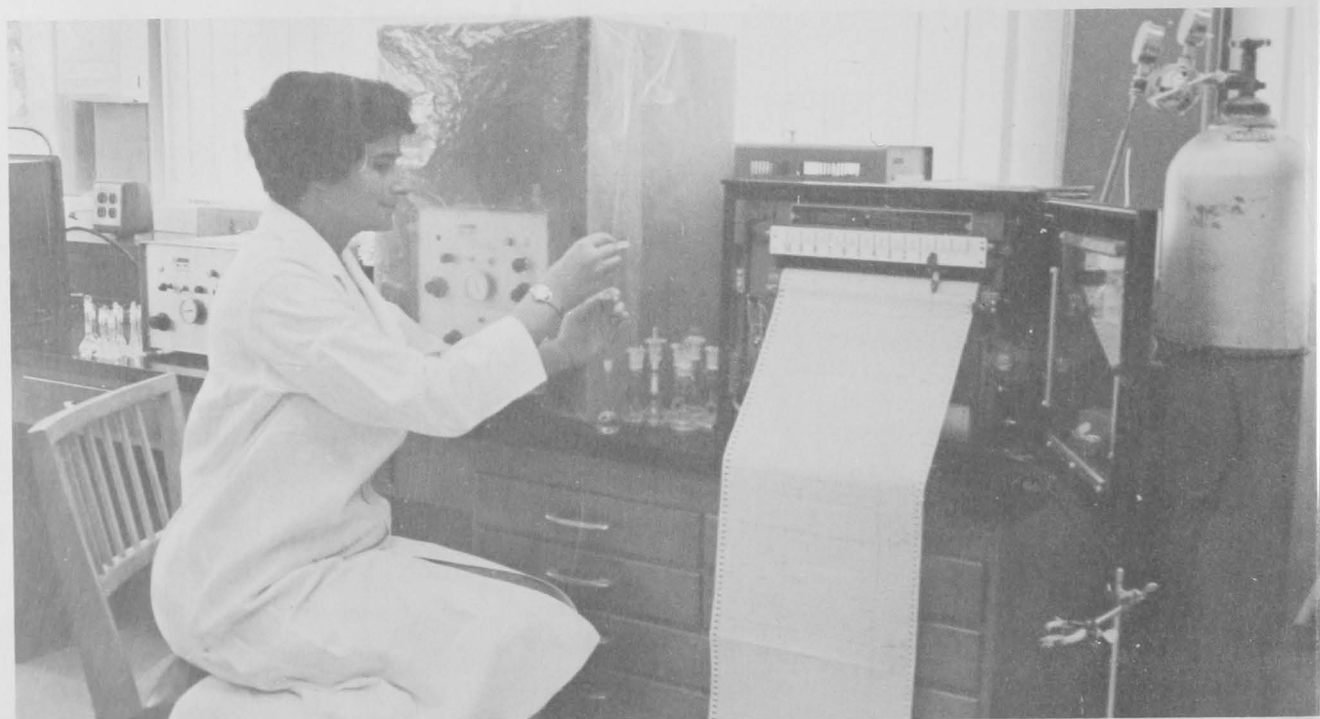
Figure 11.--Gas chromatographic analysis of pesticide residues in fishery products; identification and measurement of individual residues.
