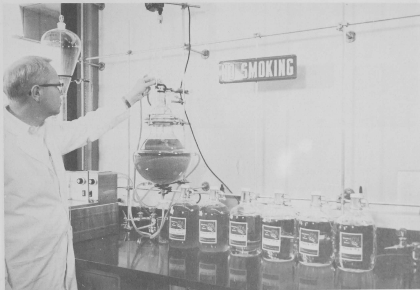
Figure 7.--Controlling temperature during a six-stage countercurrent solvent extraction of ground hake.
