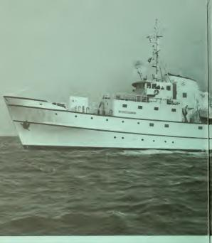
The Albatross IV, commissioned in May 1963, was especially designed for fishery-oceanographic research in the northwesterm Atlantic. This 187-foot steel stern trawler is equipped with special fishing gear and modern electronic devices including a
