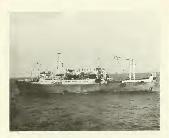
Soviet BMRT factory trawler fishing for ocean perch along Aleutian Islands. This class of trawler is equipped with processing facilities and is able to operate as an independent unit.
