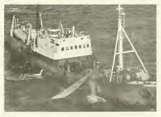
Soviet SRTM freezer trawler fishing for shrimp near the Shumagin Islands in the Gulf of Alaska. The cod end of the trawl being brought aboard the SRTM has several hundred pounds of shrimp. This class of trawler has facilities for sharp freezing and refrigerated storage and has been the mainstay of the Soviet shrimp fishing fleet off Alaska.
