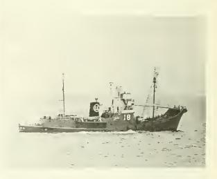
Japanese whale killer vessel hunting in the Gulf of Alaska. Killer vessels hunting for whales range many miles from the factory ship. The whales are killed by harpoons shot from guns on the bow of the killer vessels, inflated with air, and buoyed with radar reflectors or radio transmitters for retrieval by the factory ships.
