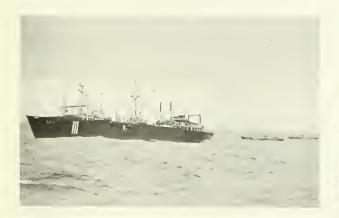
Japanese factory ship and two of her accompanying trawlers in the eastern Bering Sea. The trawlers' catches of groundfish are delivered to the factory ship primarily for production of fish meal and oil and minced fish meat.
