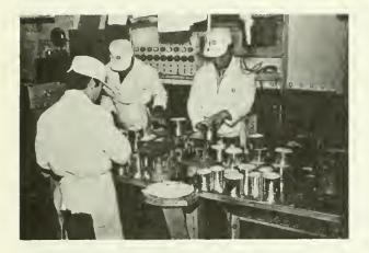
Cans of hand-packed king crab meat being checked for appropriate weight on Japanese factory ship in eastern Bering Sea. Inspected cans are conveyed to next compartment where they are sealed and then cooked in retorts.
