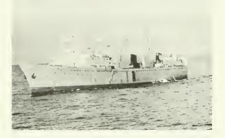
Japanese factory trawler fishing for ocean perch in the Gulf of Alaska. Japanese factory trawlers are equipped with complete facilities for processing and refrigerated storage, which enable them to operate as independent units.
