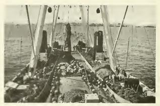
Emptying trawl on Japanese factory trawler off Kodiak Island in Gulf of Alaska. The cod end of the trawl is raised above deck, and the fish go through a hatch at the top of the stern ramp and then directly to the processing facilities below deck.
