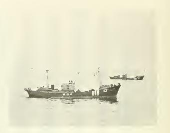
Japanese pair or bull trawlers fishing for groundfish in the eastern Bering Sea. The two vessels tow one trawl by means of a cable from the stern of each ship. These two vessels belong to a fleet of trawlers accompanying a factory ship which processes their catches.
