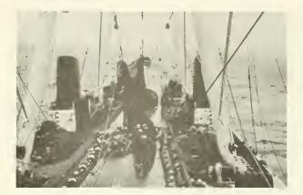
Cod end of a trawl containing several tons of ocean perch coming aboard Japanese factory trawler in Gulf of Alaska. The trawl is taken aboard via a stern ramp. The large after deck of Japanese factory trawlers provides space for carrying extra gear for repairing trawls.
