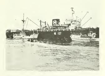
Japanese salmon factory ship with gill net vessels alongside. Each day a fleet of about 30 gill net vessels delivers its catch to a factory ship for processing.
