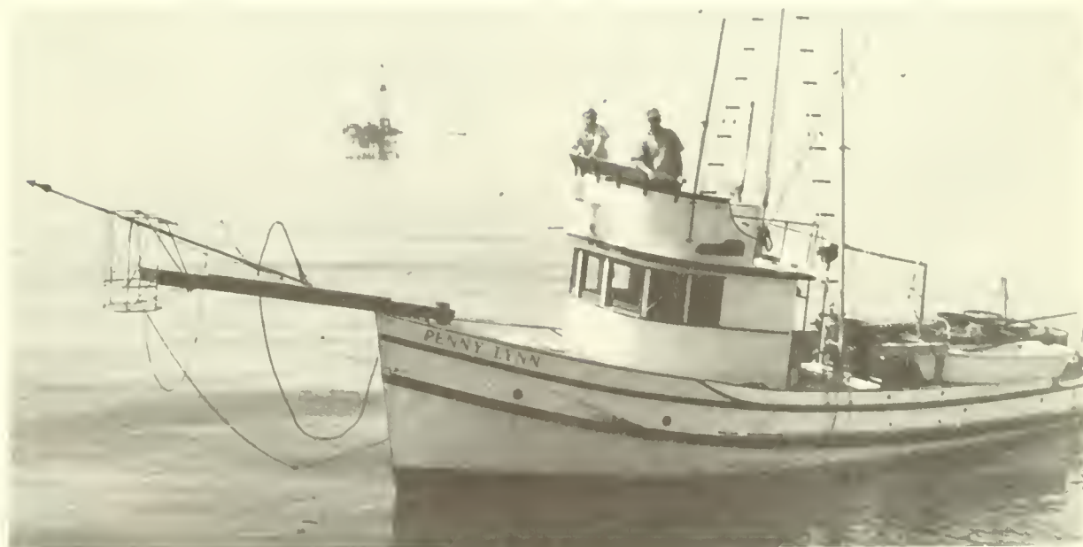
Fishing operations research—small swordfish vessel equipped with harpoon gear, now turning to basking shark fishery in off-season.
