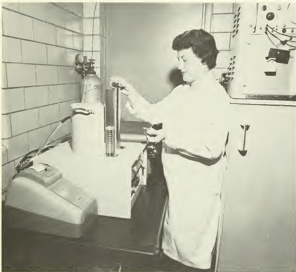
Figure 7.--The rate at which carbon is converted into organic matter by marine phytoplankton--primary production--can be measured by use of carbon 14. Investigator is preparing to analyze phytoplankton cells for their carbon 14 content with a gas-flow proportional detector equipped with an automatic sample changer.
