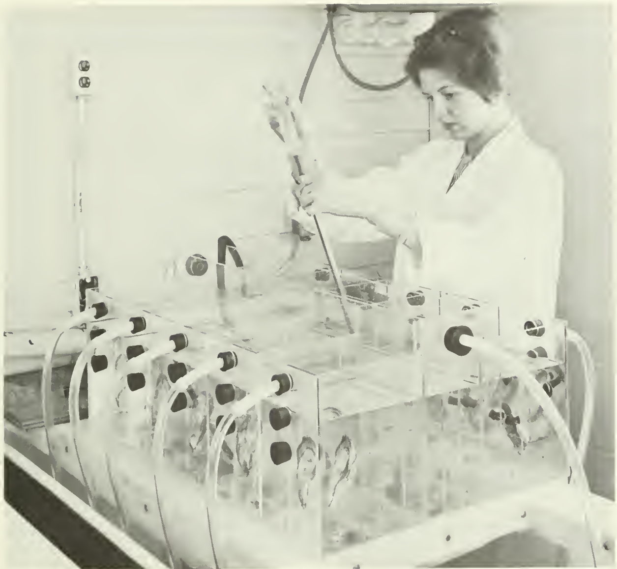
Figure 2.--Oysters, which can be seen through the clear sides of a modified "Lund" trough, are held in individual compartments and can be fed selected diets of radioactive foods. In such a system, an oyster's preference for certain species of phytoplankton can be accurately determined, along with its ability to digest and utilize them.
