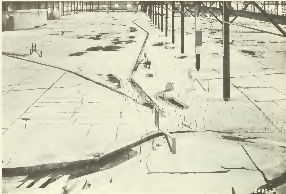
Figure 19.--The Galveston Bay model constructed by Corps of Engineers at Vicksburg, Miss., that will be used to test proposed plans for hurricane protection. (Galveston, Tex., is located at bottom of picture. Note the Houston Ship Channel extending the entire length of the dewatered model and the Texas City Channel extending from the center to the left, upper-central margin.)
