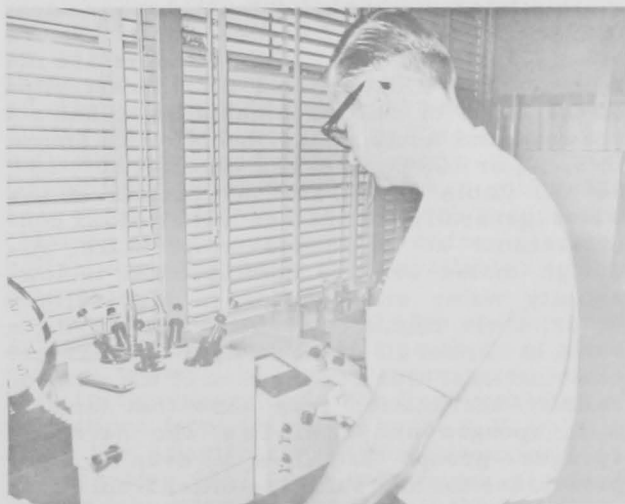
Figure 6.--Worker using a vapor pressure osmometer to determine the total osmotic concentration of the blood of blue crabs maintained at different salinities.
