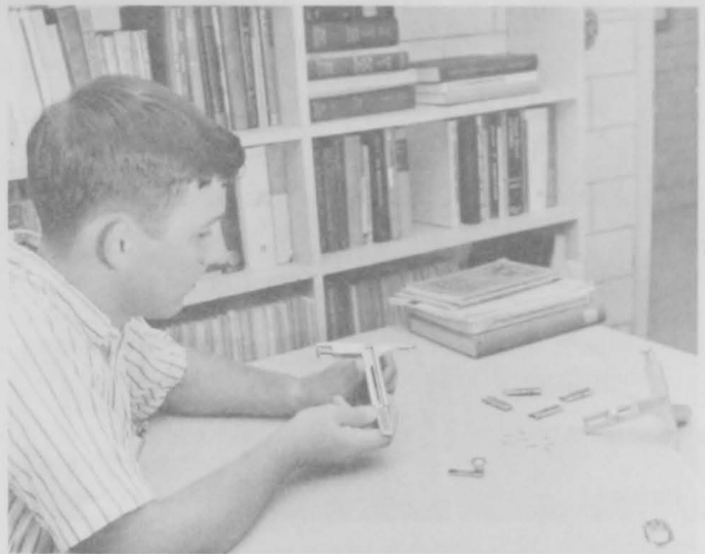
Figure 16.--Tagging "gun," showing tags in the magazine and one tag as it leaves the gun during insertion in the fish.
