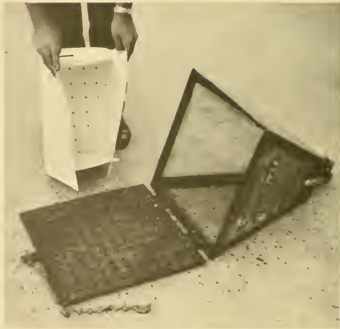
Figure 15.--Two types of containers used to transport stained shrimp to the sea floor. The disposable container now in use is on the left. When the block of salt dissolves, the container springs open.
