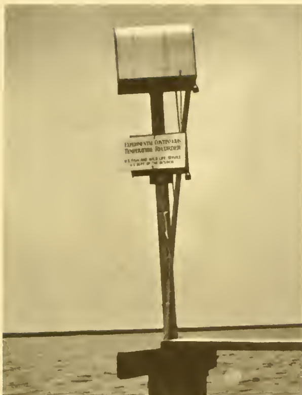
Figure 17.--Recording device measures continuously the temperature of surface and bottom waters and bottom sediments to provide information to help understand the behavior of estuarine animals.
