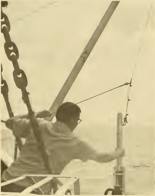
Figure 7.--Worker obtaining a temperature record with a bathythermograph before a longline set.
