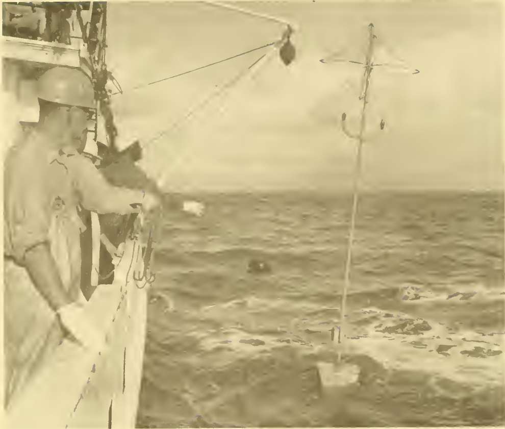
Figure 8.--The start of retrieving a longline set. Man at rail holds grappling hook to catch line attached to buoy to start the haulback.
