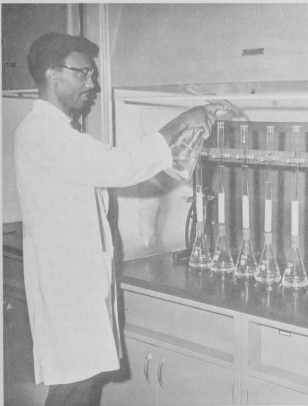
Figure 3.--The analysis of pesticide residues requires meticulous preliminary "cleanup" or removal of extraneous material from the samples.
