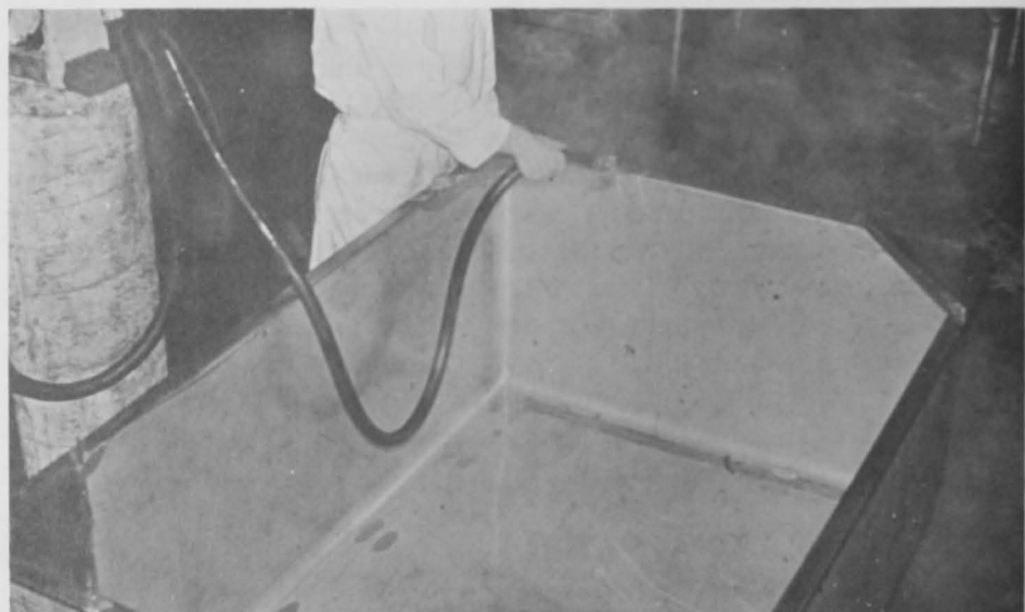
Figure 9.--All containers and utensils used for handling and processing fish should be constructed of noncorrosive materials that make cleaning easy and effective.
