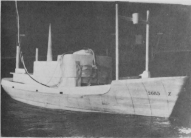
Figure 9.--Wooden model (1/16 scale) undergoing seakeeping tests.
