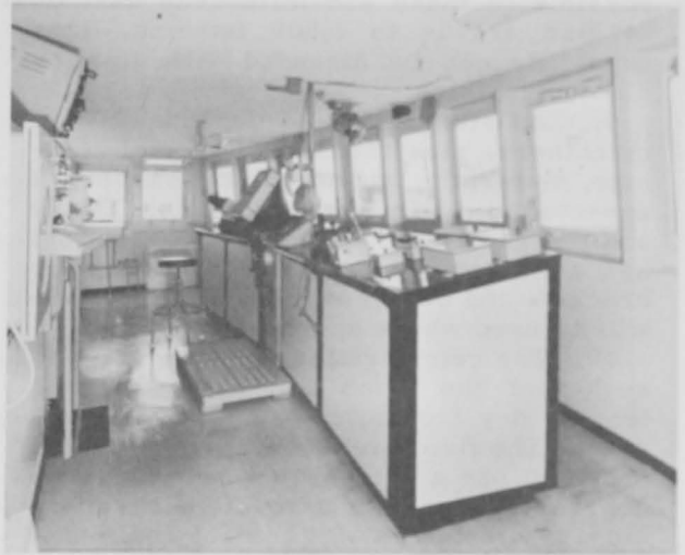
Figure 10.--Ship control console--fish detection equipment is located to port of steering wheel and ship control and navigation equipment to starboard.
