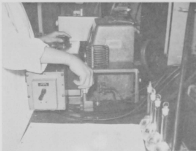
Figure 2.--Analysis of trace minerals in fish by flame photometry.
