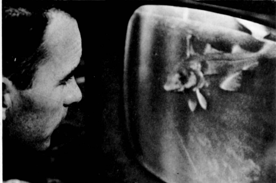
Closed circuit TV screen showing haddock. Camera is on bottom of net.
