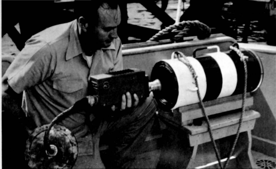
Camera unit, RCA ITV-5, is inserted into watertight housing.
