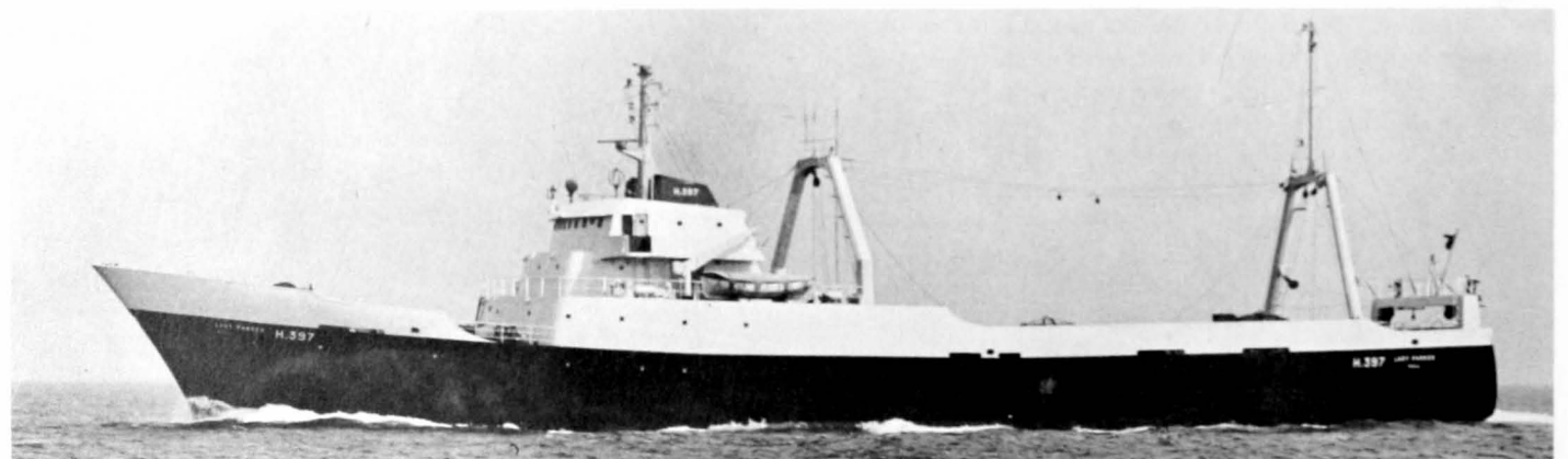
New 240-foot, all-freeze, over-the-stern-part factory trawler.
