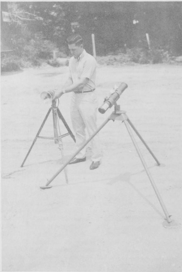
Figure 38.--Underwater TV system with tripod mounted camera and floodlight.
