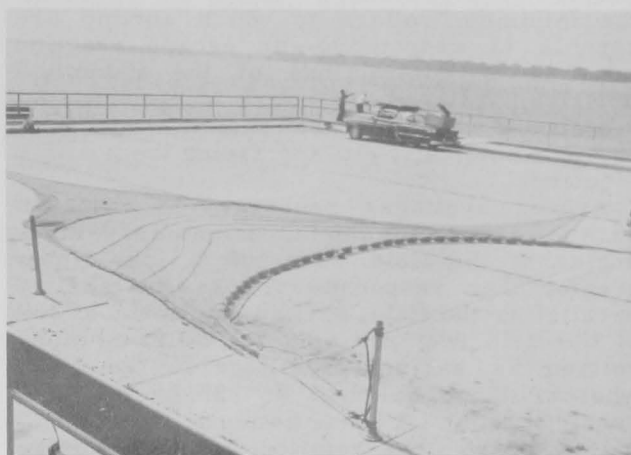
Figure 33.--An electrical shrimp trawl equipped with mud rollers. Four transverse electrodes are visible ahead of the trawl footrope.
