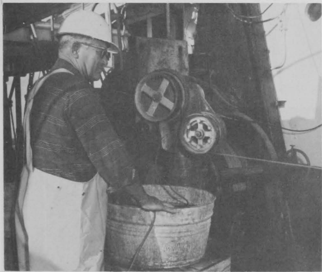
Figure 26.--The longline hauler coils the mainline neatly into the tub.
