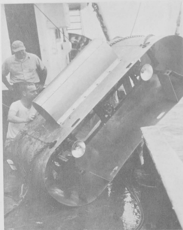
Figure 44.--CA-8 camera sled. Lithium float in housing on top.
