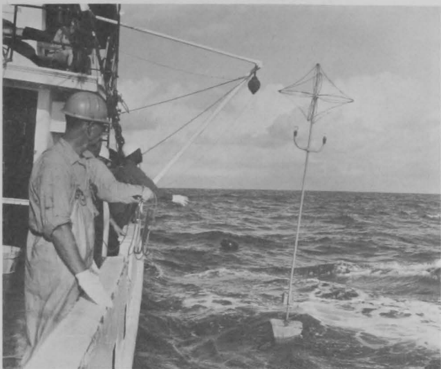
Figure 25.--Retrieval of the radar-light buoy marks the beginning of the haul-in operation of the longline set.
