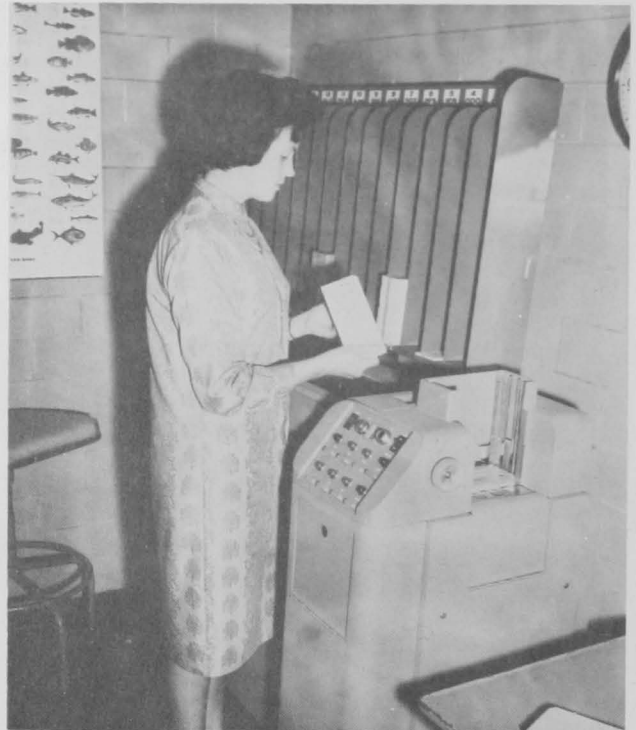
Figure 18.--High-speed card sorter used at Pascagoula.
