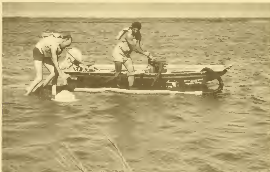
Figure 34.--New "vacuum cleaner" bottom sampler being tested. This device provides a quantitative sample by removing all sediments and animals from 1/10 m. 2 (1.08 ft. 2 ) of the bottom to a depth of 5 in.
