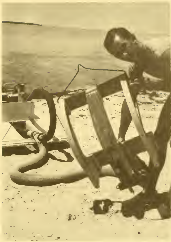
Figure 12.--Sled with suction head affixed between parallel guides.
