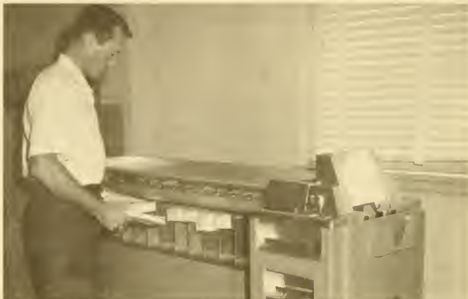
Figure 25.--Sorting ADP Cards for computer analysis. All data collected in the estuary during 1963 and 1964 have been transcribed to more than 250,000 cards to facilitate their storage, retrieval, tabulation, and analysis.
