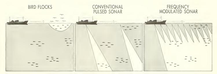
FIGURE 7. The new continuous-transmission, frequencymodulated sonar to be installed aboard the *Townsend Cromicell* will allow scientists to track individual fish and fish schools underwater. To locate tuna schools the commercial fleet now depends heavily on sighting bird flocks.
