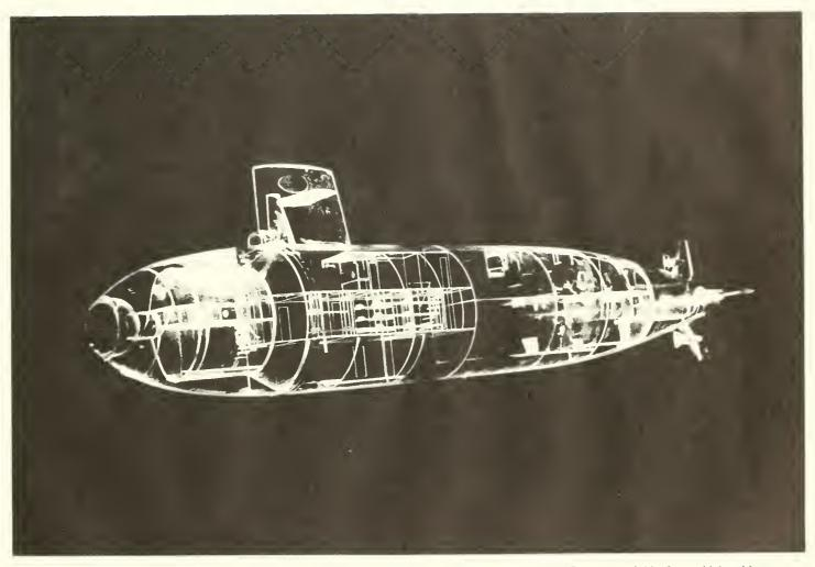
FIGURE 27. Plastic model of nuclear-powered submarine proposed by this Laboratory for fishery-oceanography research. The eraft would be 163.5 feet long and carry a scientific party of 7, a rrew of 24. It would be able to make a host of studies impossible to carry out from surface ships. tinuous environmental sampling, and quiet operation are also essential.
