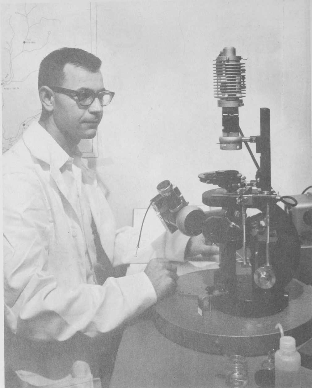
Figure 18.--Inverted plankton microscope with attachments for microphotography.
