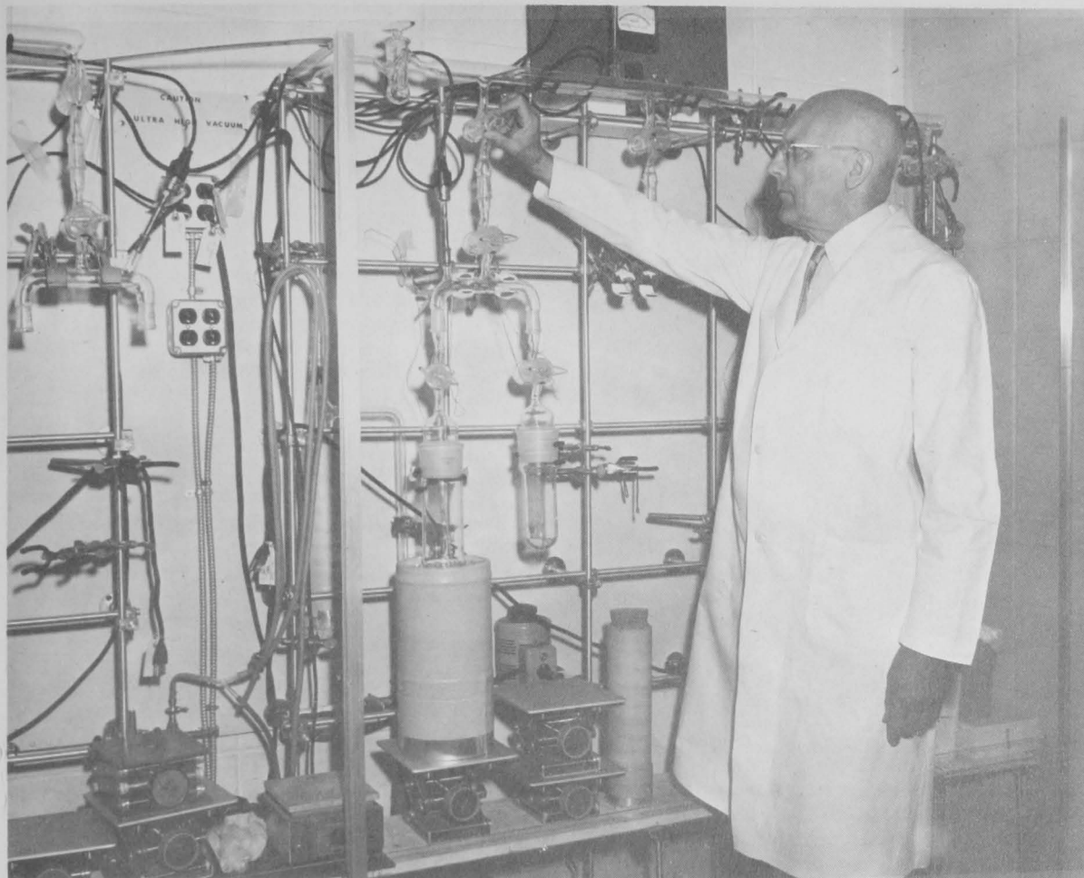
Figure 13.--Collection of the volatile components from fishery products by a high-vacuum, low-temperature distillation technique.
