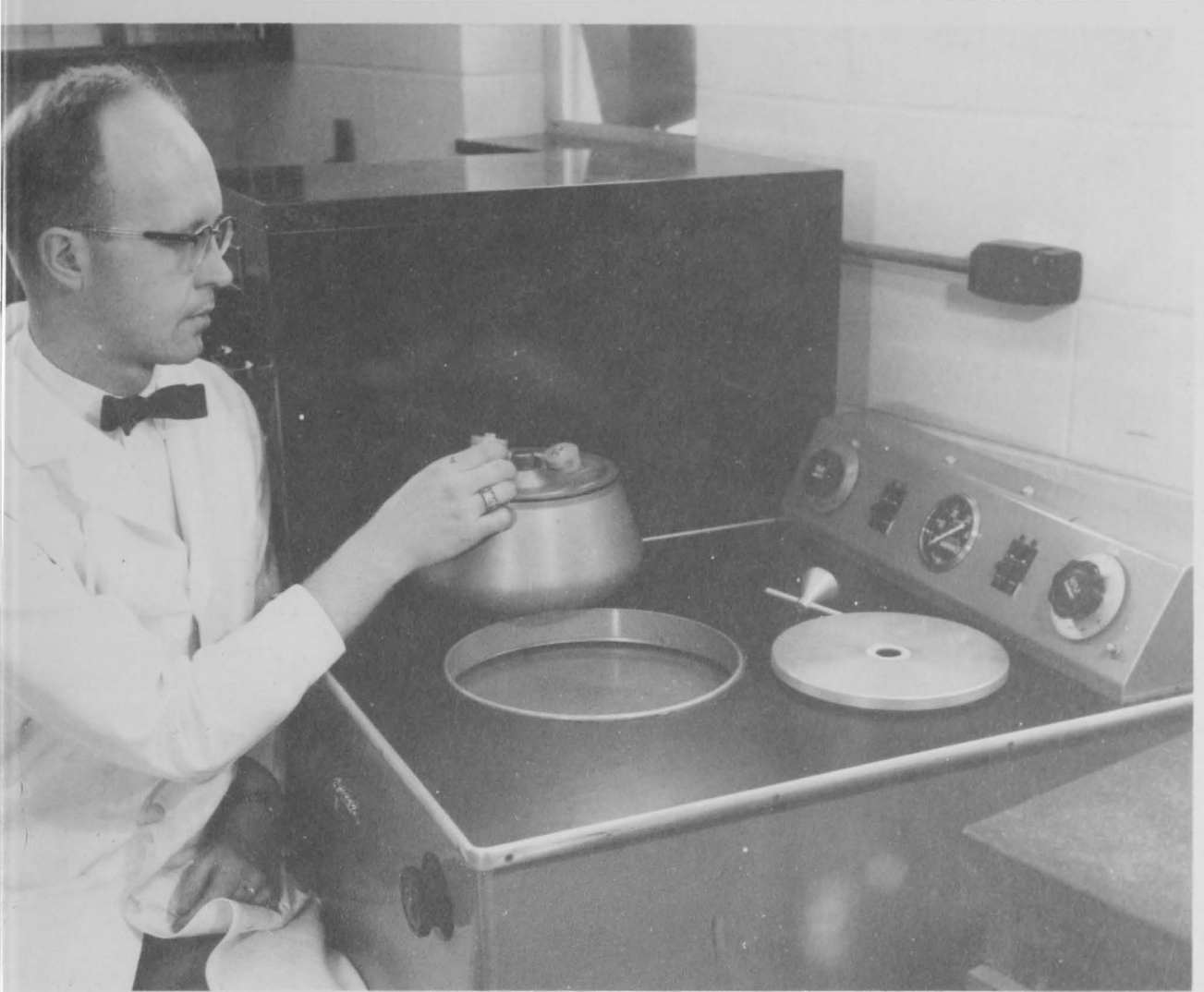
Figure 2.--Clarification of a protein extract by preparative ultracentrifugation.
