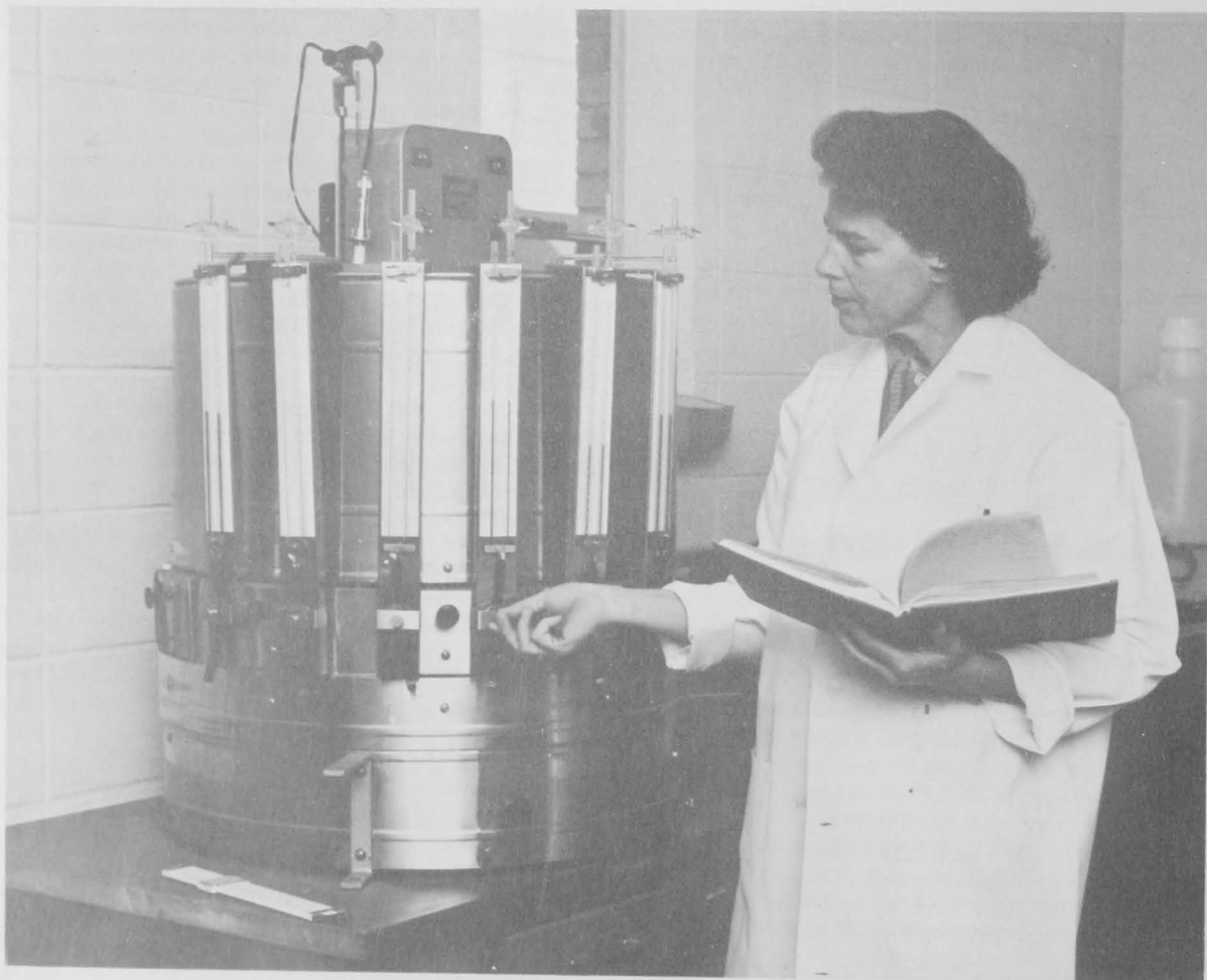
Figure 8.--This Warburg manometric apparatus is one of the tools used in the study of fish muscle enzymes, a project designed to find an objective biochemical test of quality change in frozen fish.
