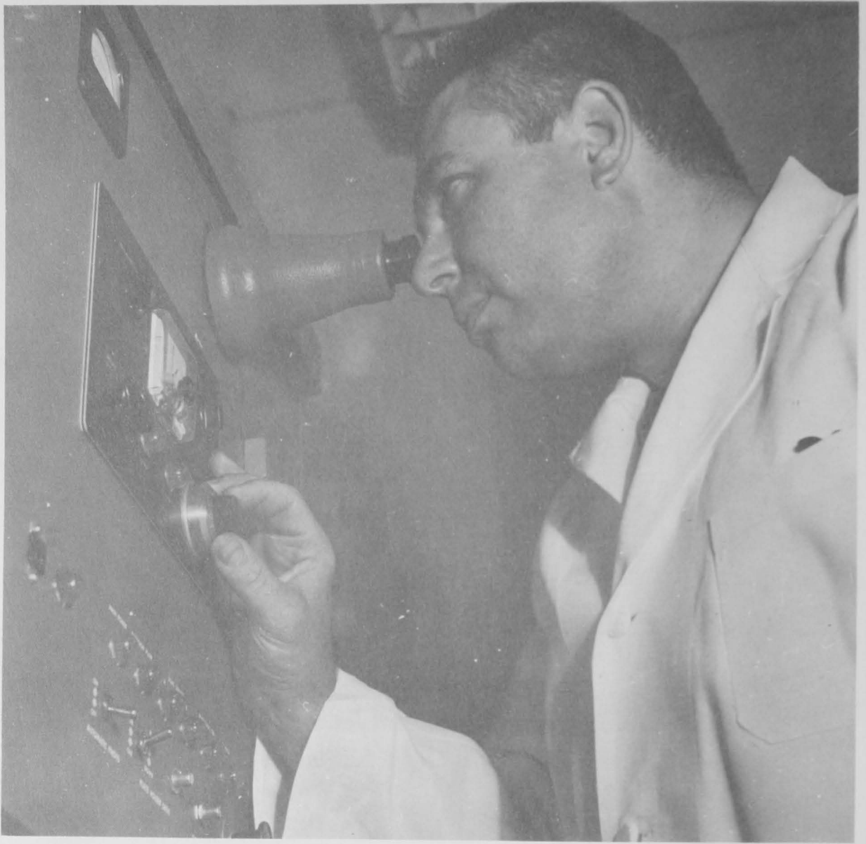
Figure 3.--Viewing the pattern of the protein components of a fish muscle extract as they are separated by the analytical ultracentrifuge.
