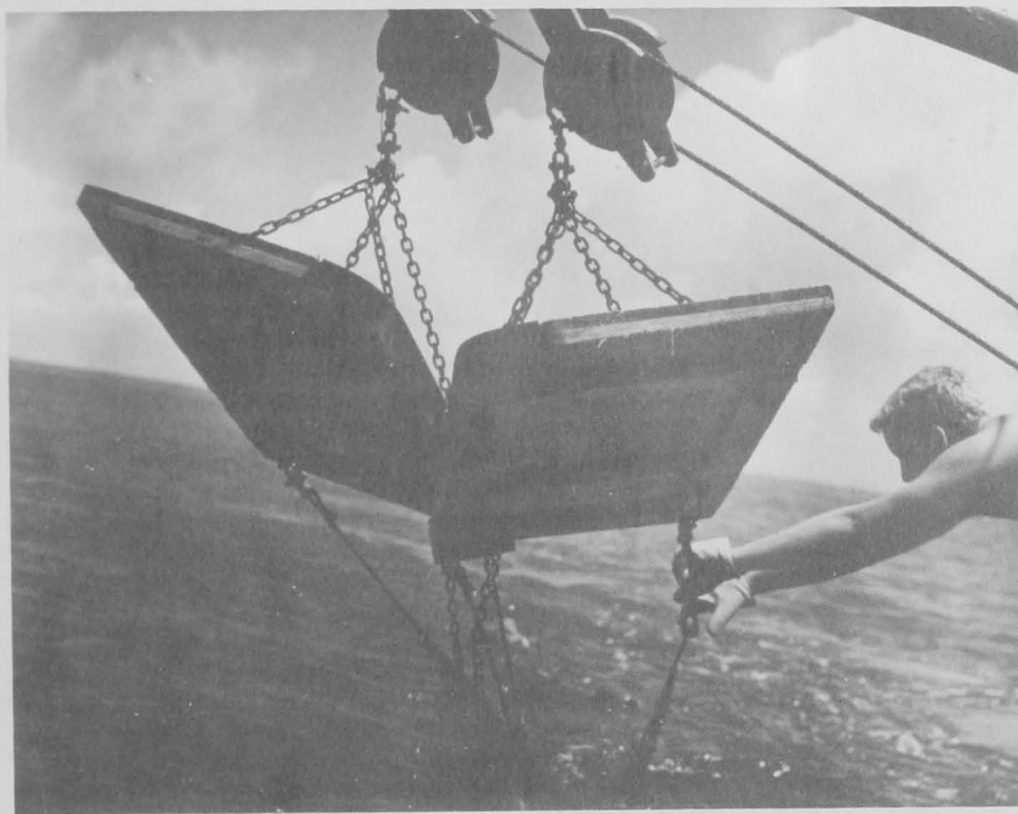
Figure 4.--Sampling for blue crabs at Drum Inlet, N.C. The 20-foot trawl is being taken aboard after a 10-minute drag.
